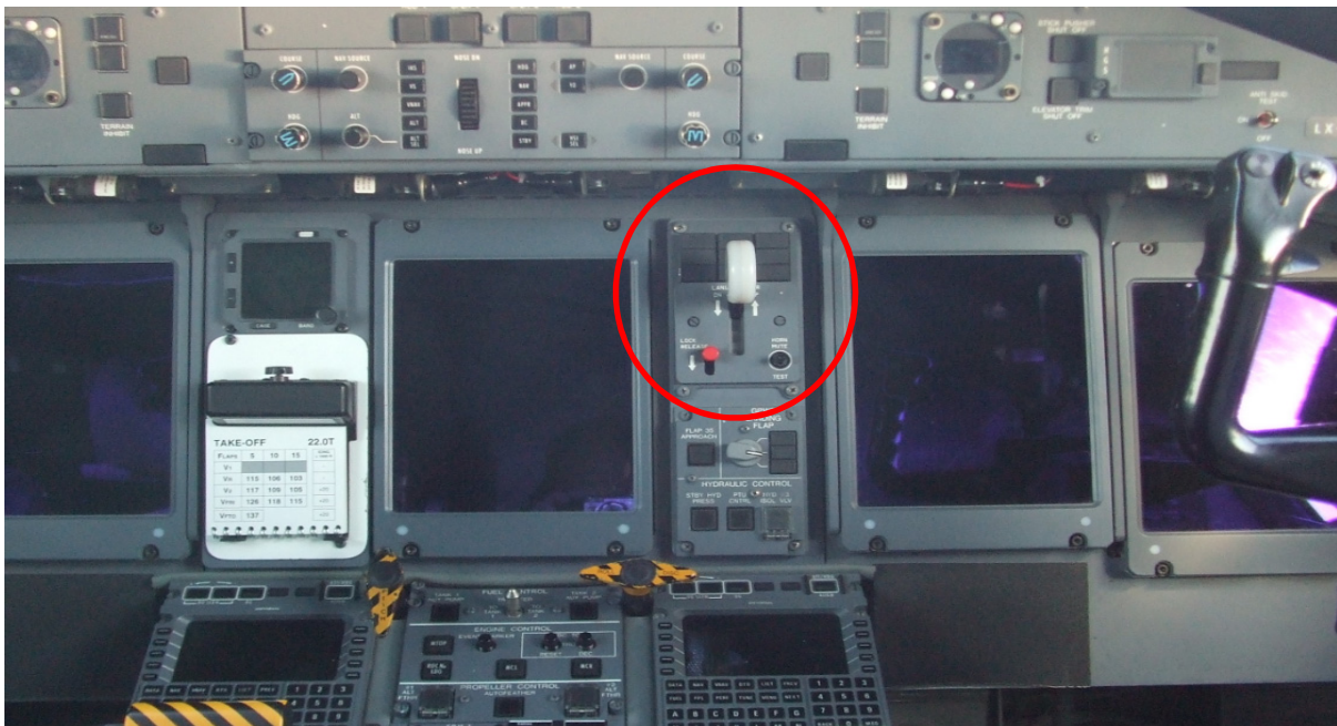
Position landing gear lever, Lock Release and indication lights in the cockpit
