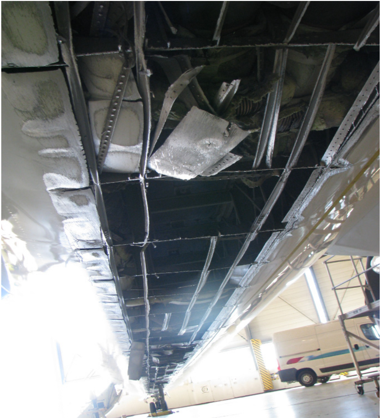
Damage on the fuselage's bottom surface (in flight direction)
