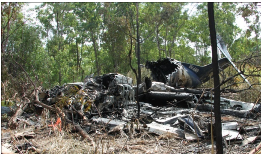
Figure 12: Aircraft wreckage, showing the extensive fire damage
