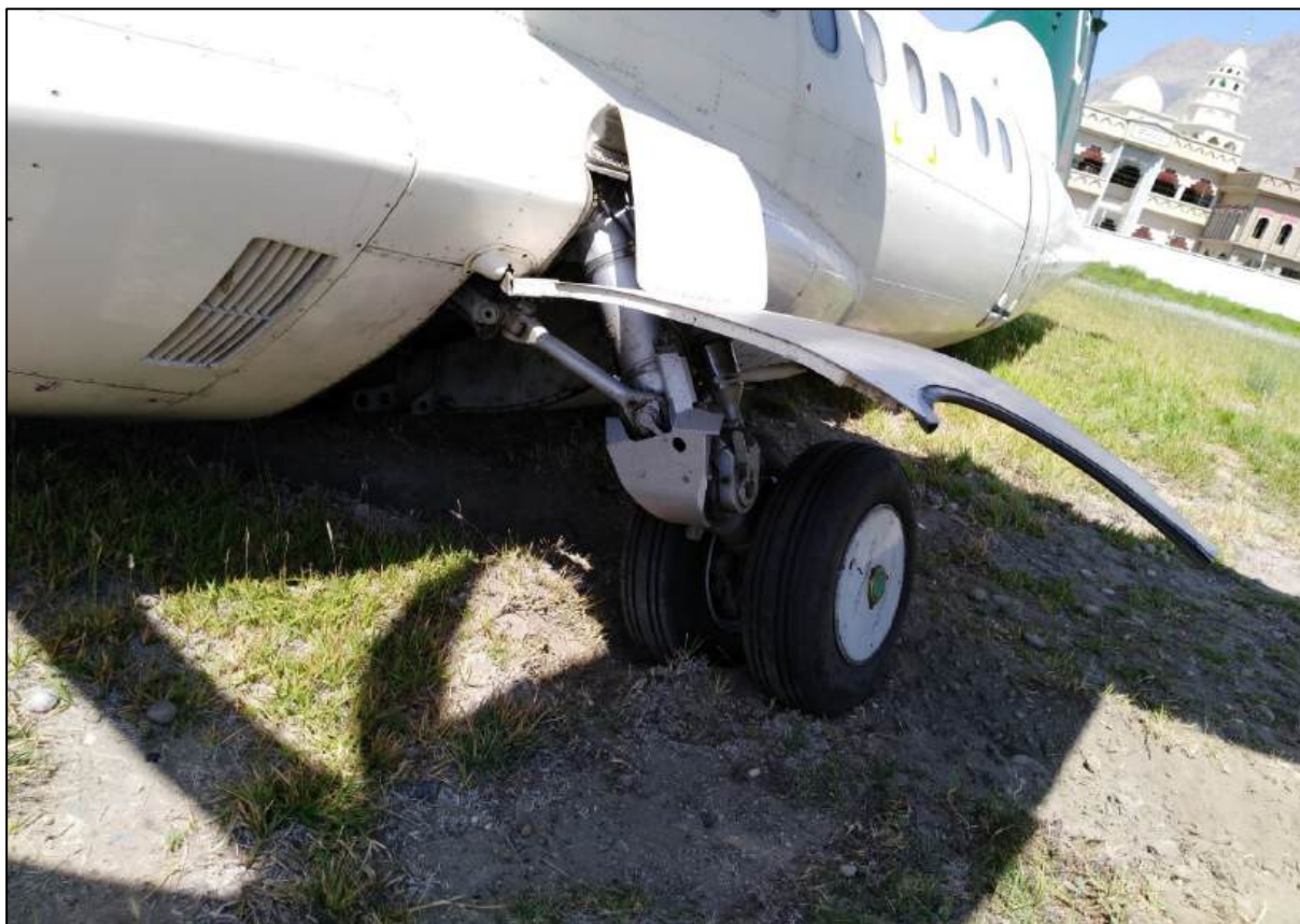
Figure 9 Left MLG damaged
