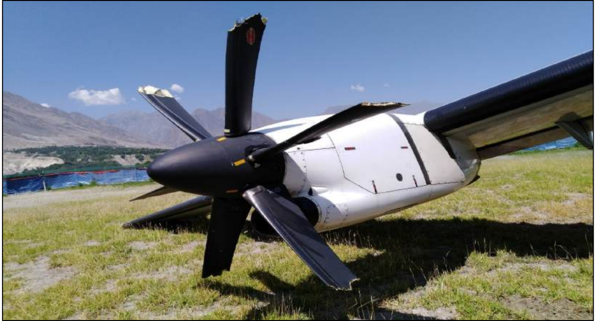
Figure 1 Broken Propellor Blades of Right Engine
