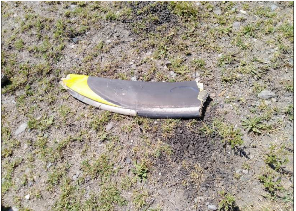
Figure 2 Broken Propellor Blade
