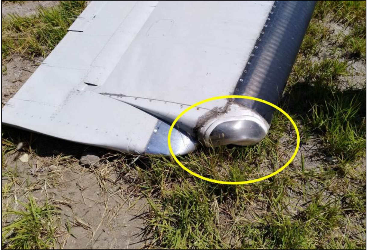
Figure 7 Right Wing Navigation Light Damaged
