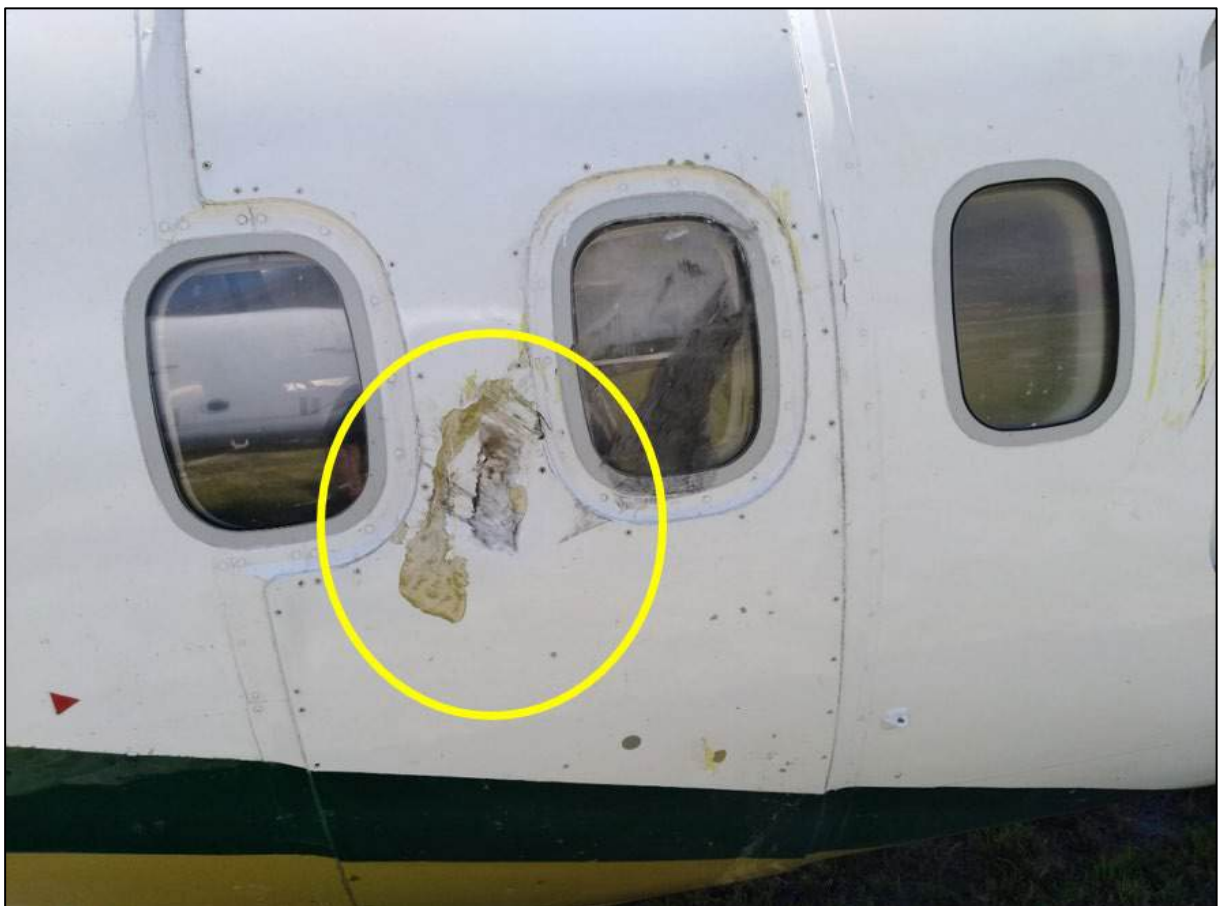
Figure 4 Impact Marks on Fuselage
