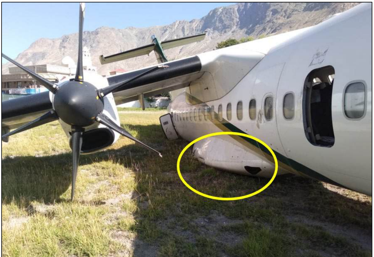
Figure 6 Right MLG Fairing Area Damaged
