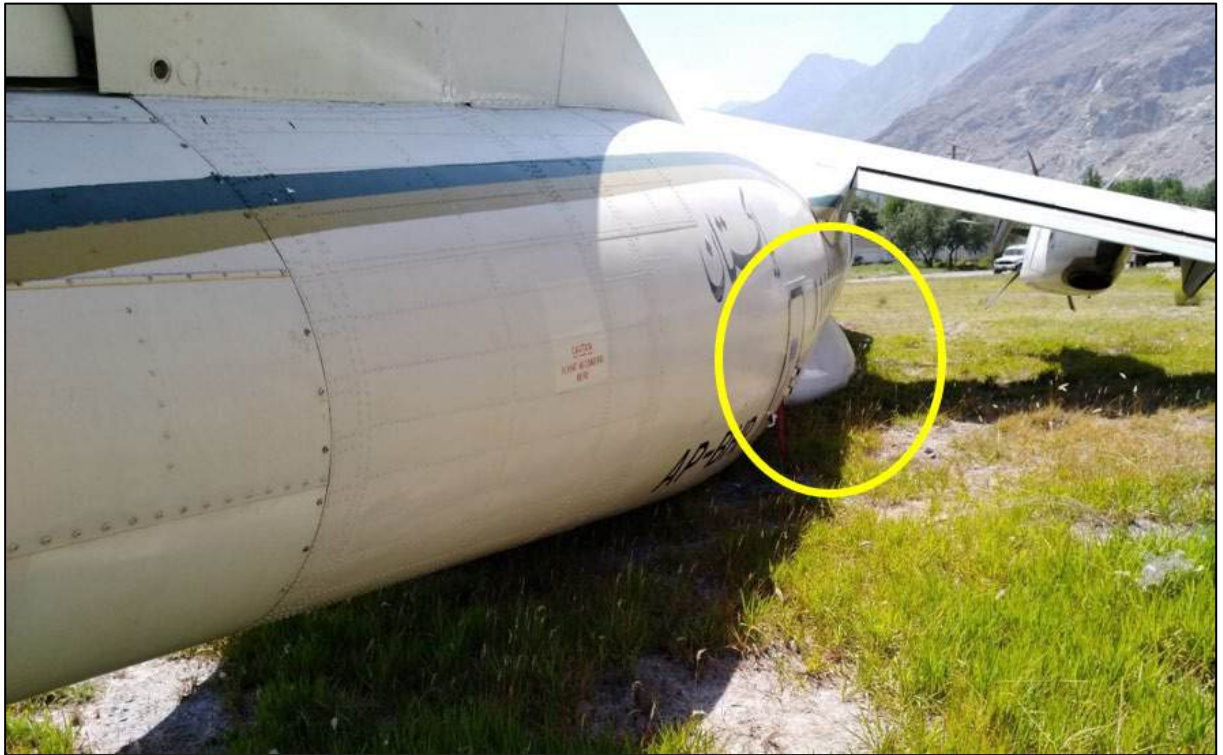
Figure 5 Right MLG Collapsed
