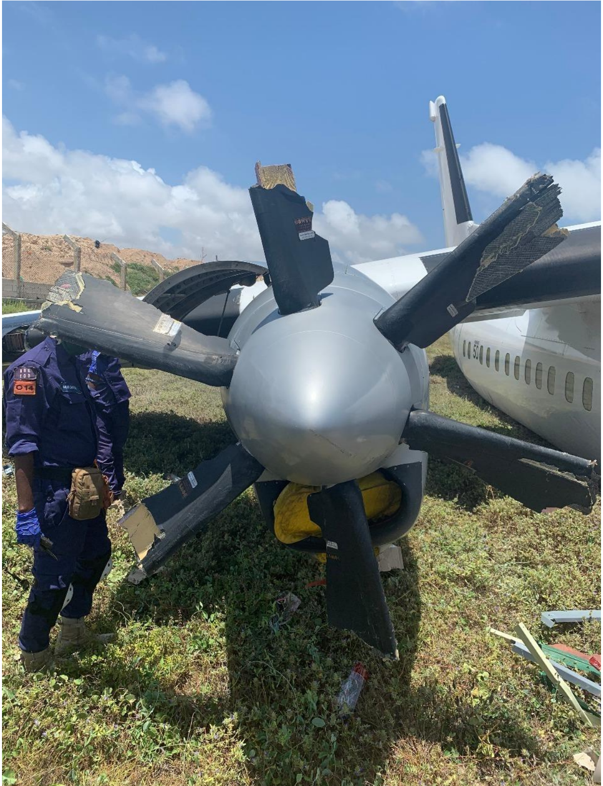
Figure 1: Propeller damage (It is evident that propeller was running which implies the engine was still functioning)
