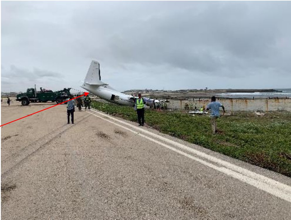
Figure 4: Aircraft veered off on the right and impacted to the perimeter wall
