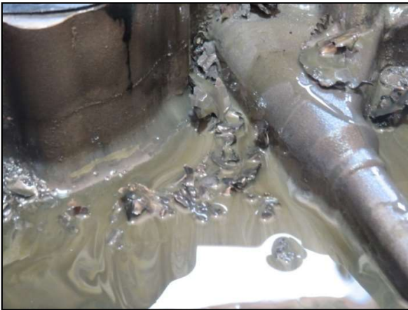
Fig 26: Broken metal pieces in Oil Sump
