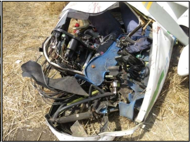
Fig 9: Front View of Badly Damaged Cockpit
