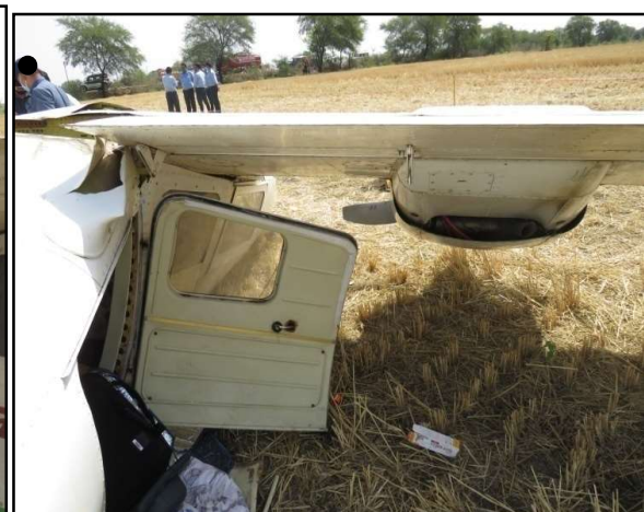
Fig19:View of Right Engine & Right Flap in Up
