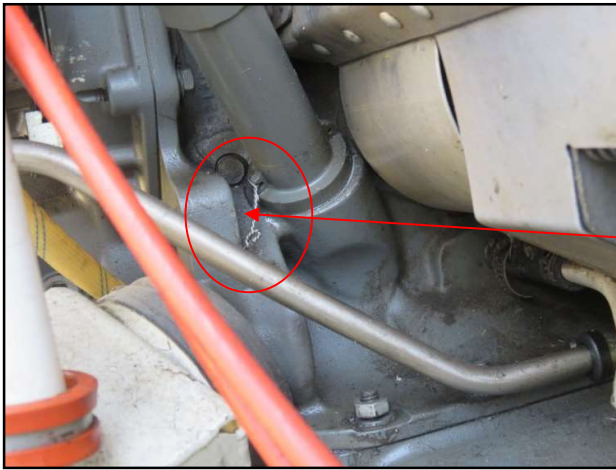
Fig 22: Oil Filler tube wire lock position
