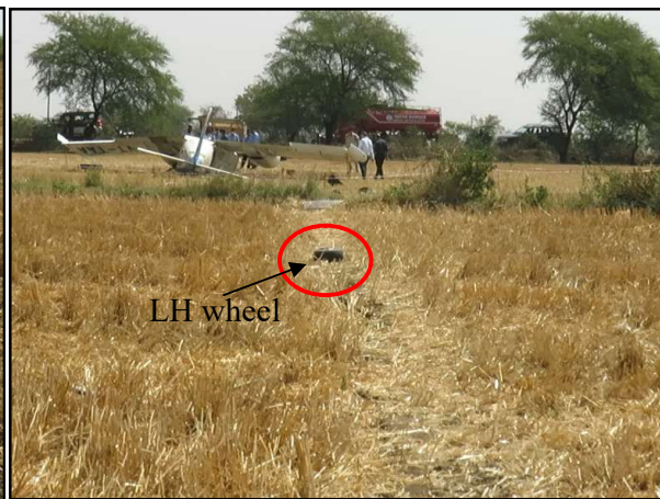
Fig 5: Dislodged wheel on field
