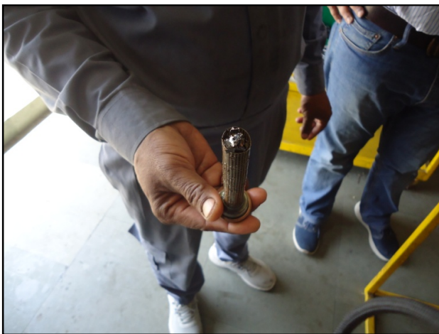
Fig 30: Suction Screen filled with Metal pieces
