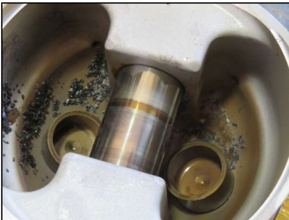
Fig 24: Metal Particles inside no 4 Piston
