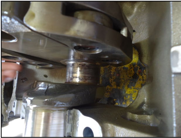
Fig 28: Abrasion marks on No 4 Crank Shaft
