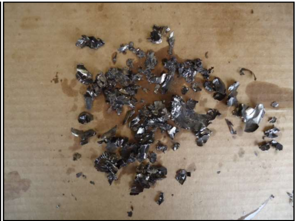
Fig 27: Metal pieces collected from Oil Sump
