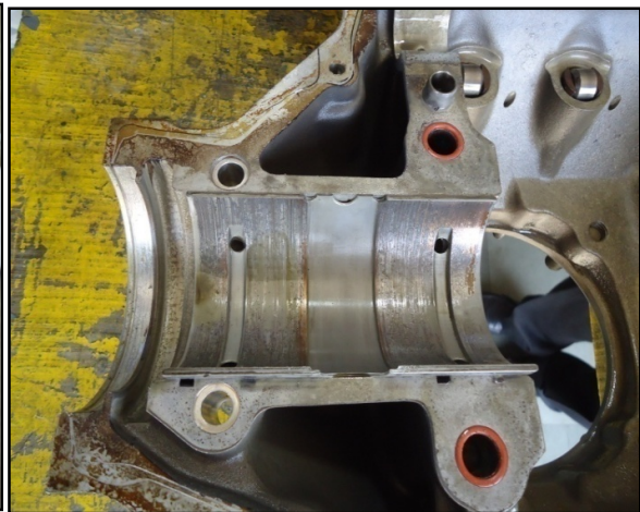
Fig 29: Scoring marks on Main bearing
