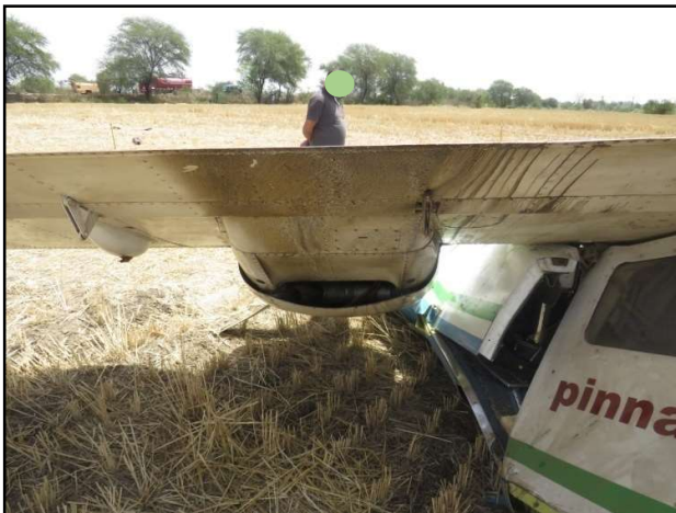
Fig18:View of Left Engine & Left Flap in Up
