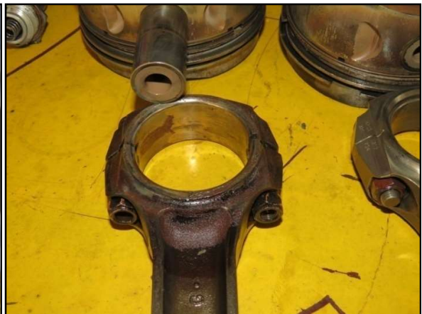
Fig 25: No 4 Piston Connecting rod without Bearing
