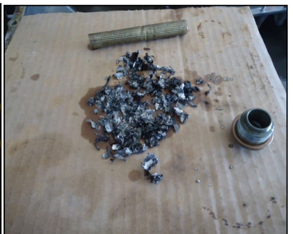
Fig 31: Suction Screen & Metal pieces
