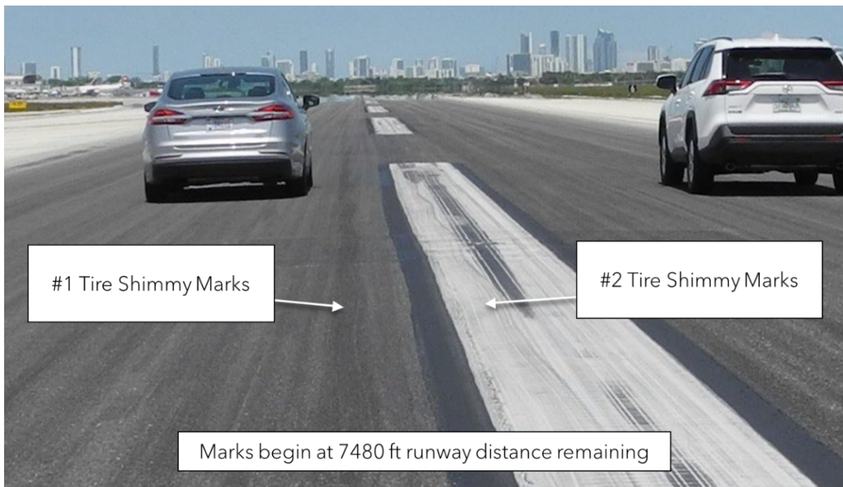
Figure 9. Start of the left main landing gear shimmy marks. The distance noted is distance to the end of the runway.
