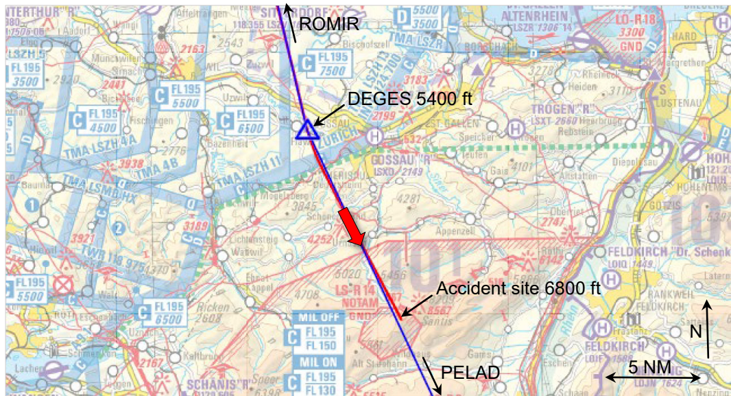
Figure 1: Planned flight path (blue) and flight path recording (red) of the D-FLIC, shown on the aeronautical map of Switzerland (source of map: Federal Office of Topography).
