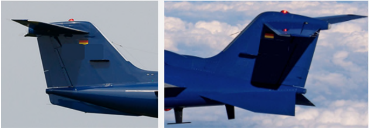
Fig. 12: Tail section of a Learjet without (original) and with Avcon Fins
