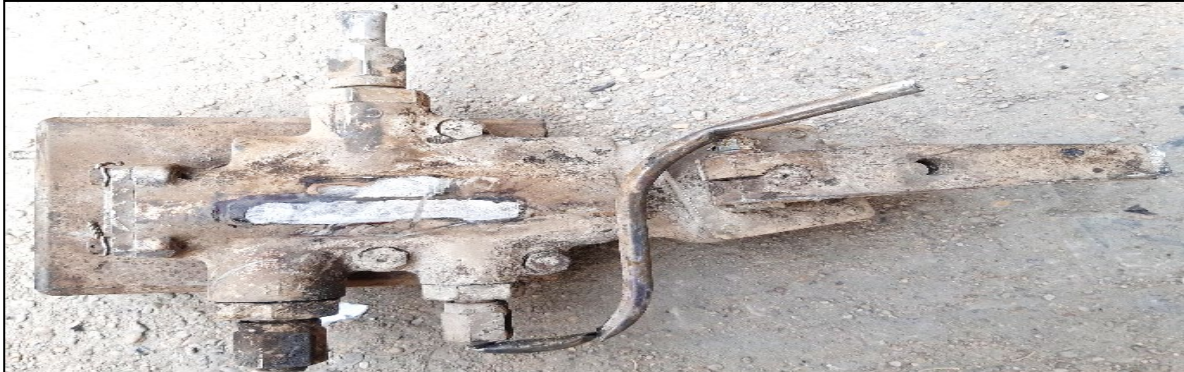
Figure 60 – MLG or NLG Vent Valve with the Free-Fall Input Lever in Position “Not Used”
