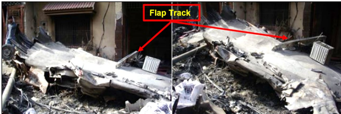
Figure 29 – R/H Wing (Rib 15 to 24) Lower Surface Facing Up and FLAP Track 4 Visible
