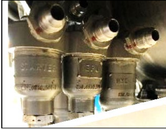
Figure 93 – Drain Collector Assembly Forward View (Undamaged)
