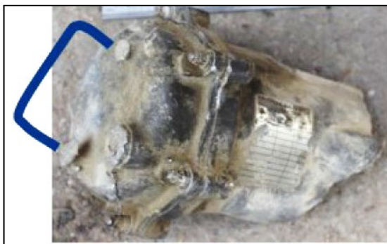
Figure 80 – Fuel Filter Cover with Missing Handle (Accident Case)
