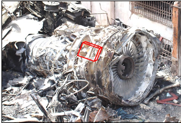
Figure 68 – ECU is Missing
