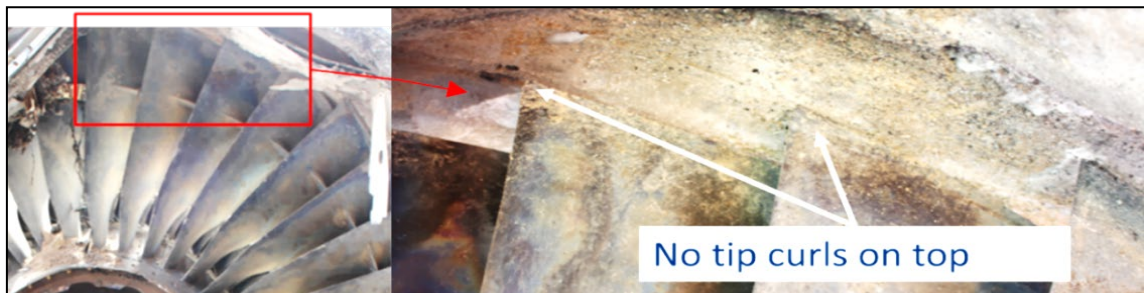
Figure 72 – Few Tip Curls, No Bent Blades. Indication of No or Low Rotation during Crash
