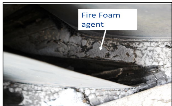
Figure 71 – Fan Blade's Fire Foam Agent Traces
