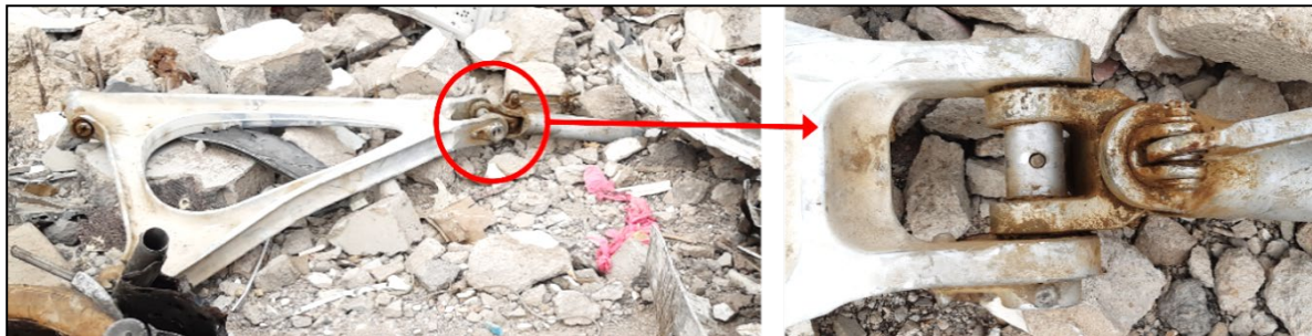
Figure 58 – NLG Drag Strut Assembly with Missing Uplock Roller
