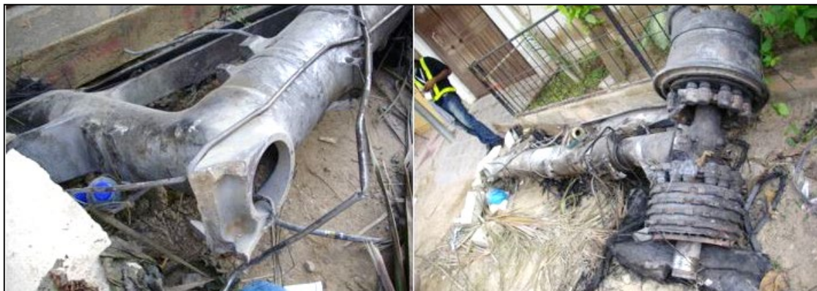
Figure 30 – L/H MLG with Missing Wheel and Tyres
