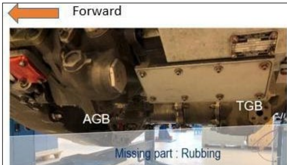
Figure 140 – TGB Missing Part
