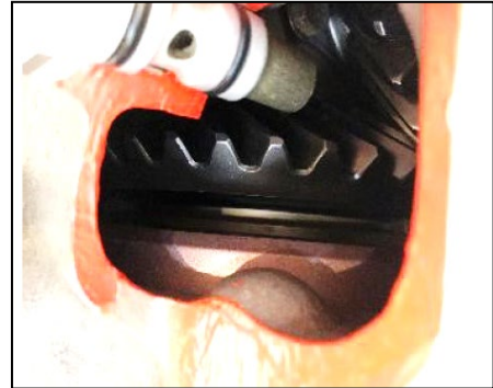
Figure 78 – TGB Conical Gear: Cut View
