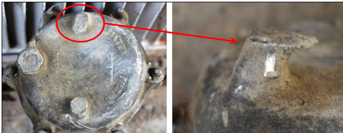
Figure 82 – Fuel Filter Cover with Missing Handle (Accident Case): Heavy Rubbing
