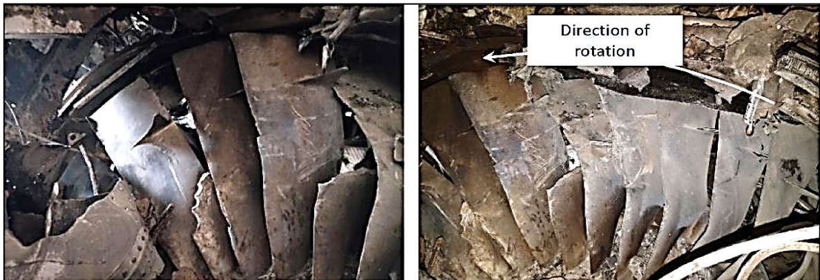
Figure 64 – Fan Blades Damaged and Bent
