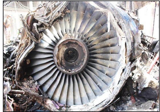
Figure 69 – Front View of Fan Blades not bent. No indication of Soft Body (i.e. birds) Impact Damage
