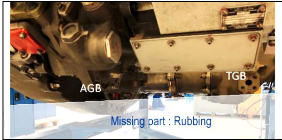
Figure 75 – Engine’s TGB and AGB with Missing Part on New Engine (in Grey Shade)
