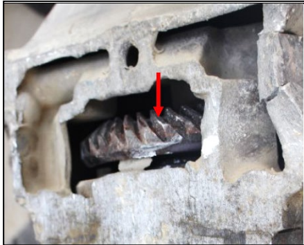
Figure 77 – TGB Conical Gear: Rubbing of the Outer End Gear Teeth: Cylindrical Shape
