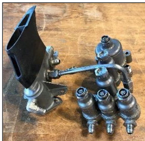
Figure 84 – Drain Collector Assembly (Undamaged)
