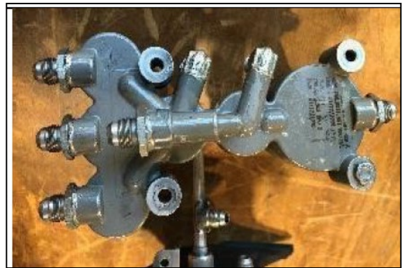
Figure 88 – Drain Collector Assembly (Undamaged)
