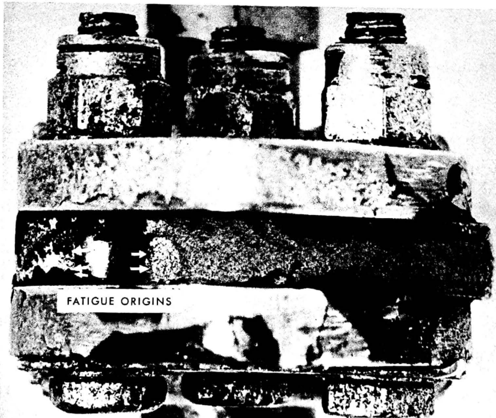
ENLARGED VIEW SHOWING FATIGUE FRACTURE
