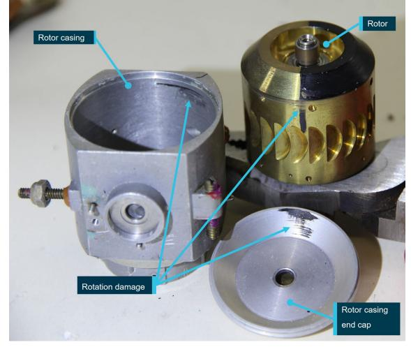
Figure 22: Left artificial horizon internal components showing rotational contact damage
