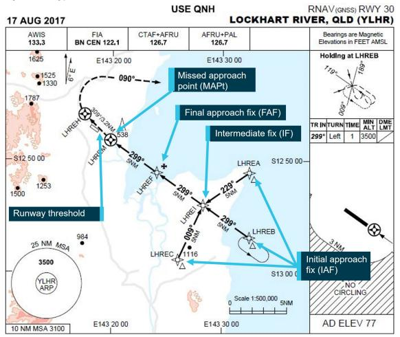
Figure 13: Extract from Lockhart River RNAV GNSS runway 30 approach chart showing layout of waypoints
