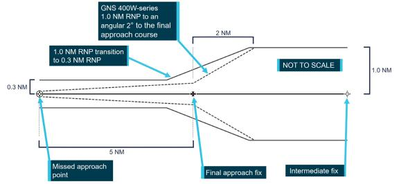
Source: ATSB, derived from information contained in ICAO Doc 8168 Procedures for Air Navigation Services-Aircraft Operations, Vol II – Construction of Visual and Instrument Flight Procedures and the Garmin GNS 400W-Series Pilot's Guide & Reference manual.
