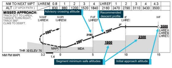
The full approach chart is provided in Figure 2. Source: Airservices Australia, annotated by the ATSB
