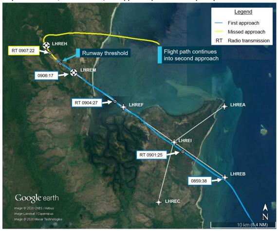
Figure 3: Flight track of VH-OZO during first RNAV GNSS approach at Lockhart River Airport with times, feature labels, and approach parameters superimposed
