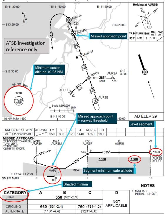
Figure 23: Extract of the Aurukun RNAV (GNSS) RWY 34 approach
