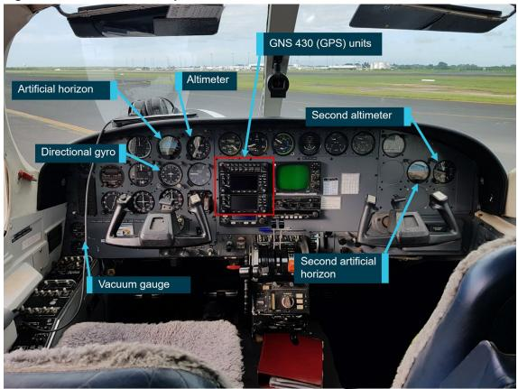
Figure 7: VH-OZO instrument panel
