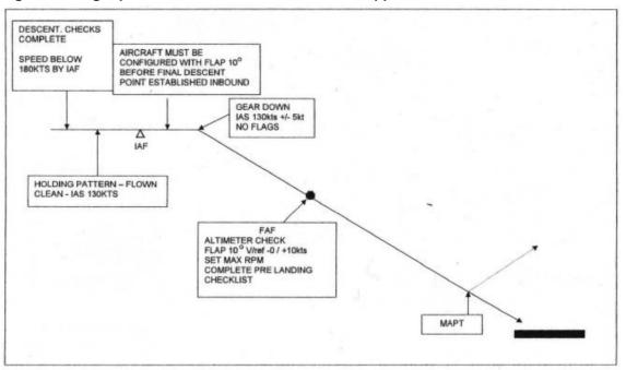
Figure 19: Flight profile for Cessna 404 RNAV GNSS approach
