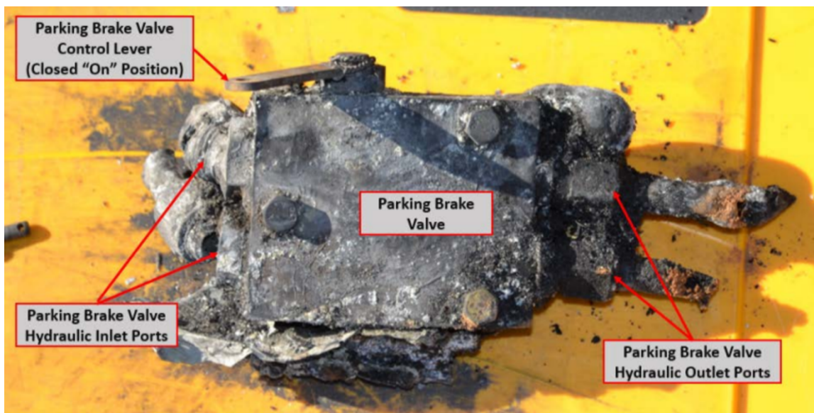
Figure 5: Parking brake valve after removal from the wreckage
