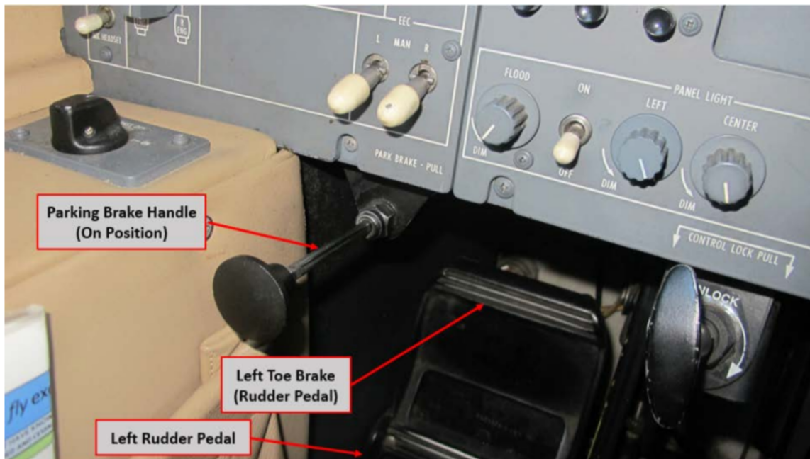
Figure 1: View of the parking brake pull knob in the ON position in reference to the instrument panel in an exemplar CE-560XL.
