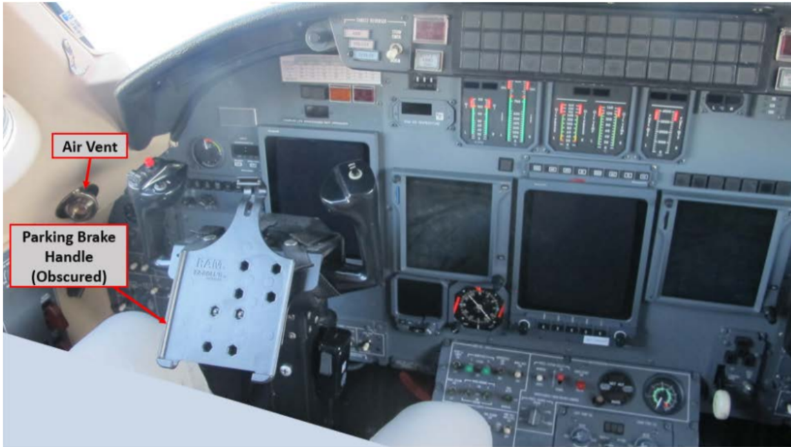
Figure 2: Location of the obscured parking brake pull knob within an exemplar CE-560XL
