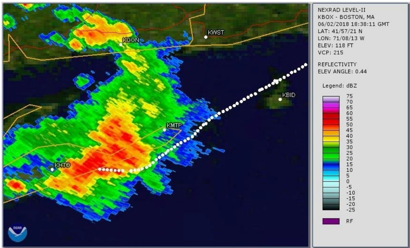
Figure 1: Boston WSR-88D Base Reflectivity Image at 1438 with flight track
