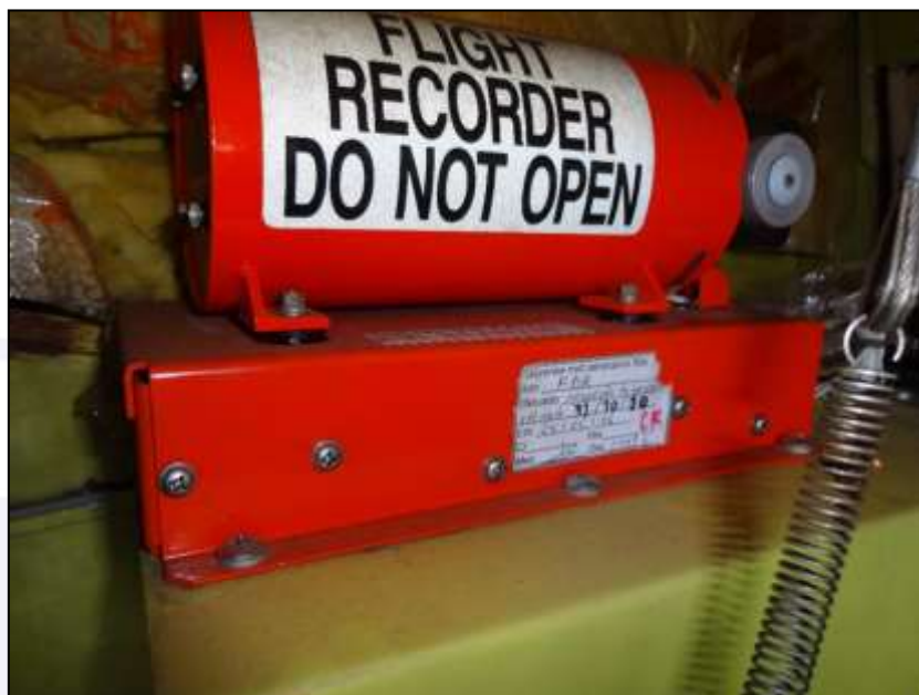
Figura 5 - Cockpit Voice Recorder CVR Honeywell, model AR-30.
