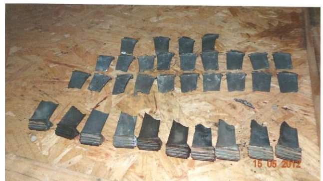
Figures 4 and 5 – General view of the power turbine rotor, and the fractured blades of this assembly.
