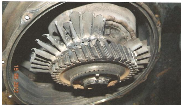
Figures 4 and 5 – General view of the power turbine rotor, and the fractured blades of this assembly.
