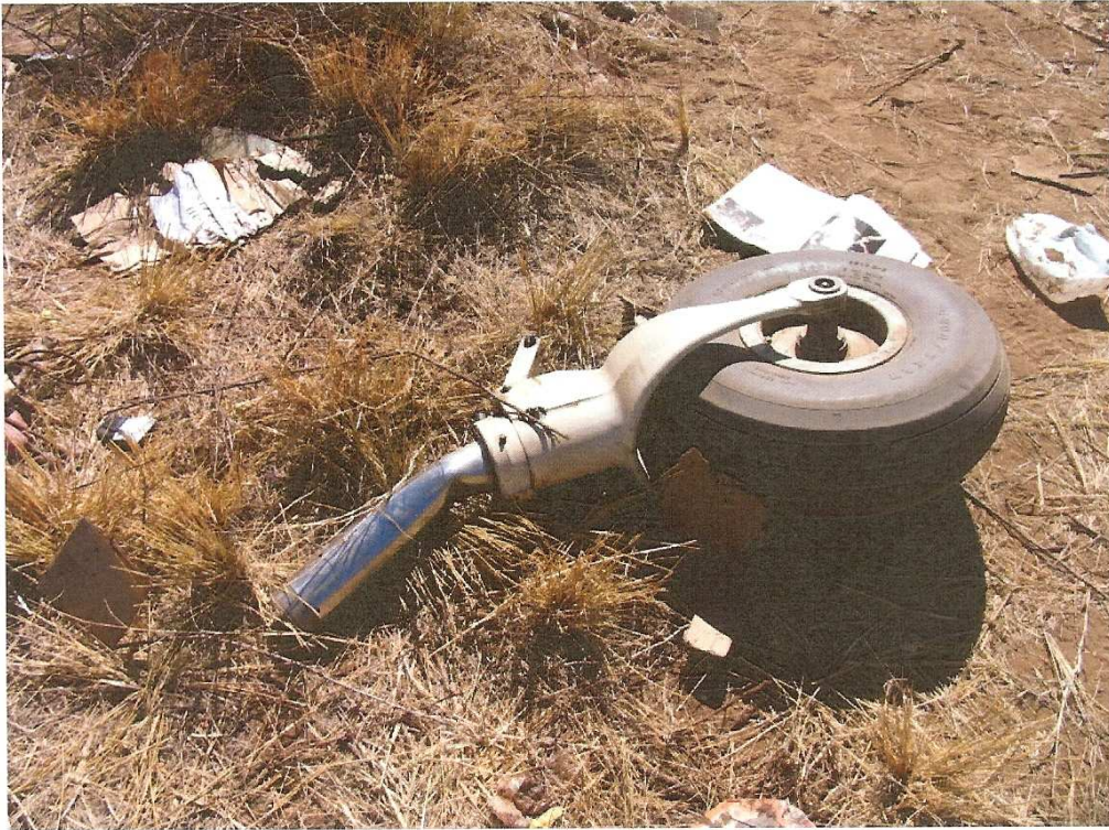
Figure 6: The nose landing gear was broken off from the aircraft and was found a distance from the main wreckage.
