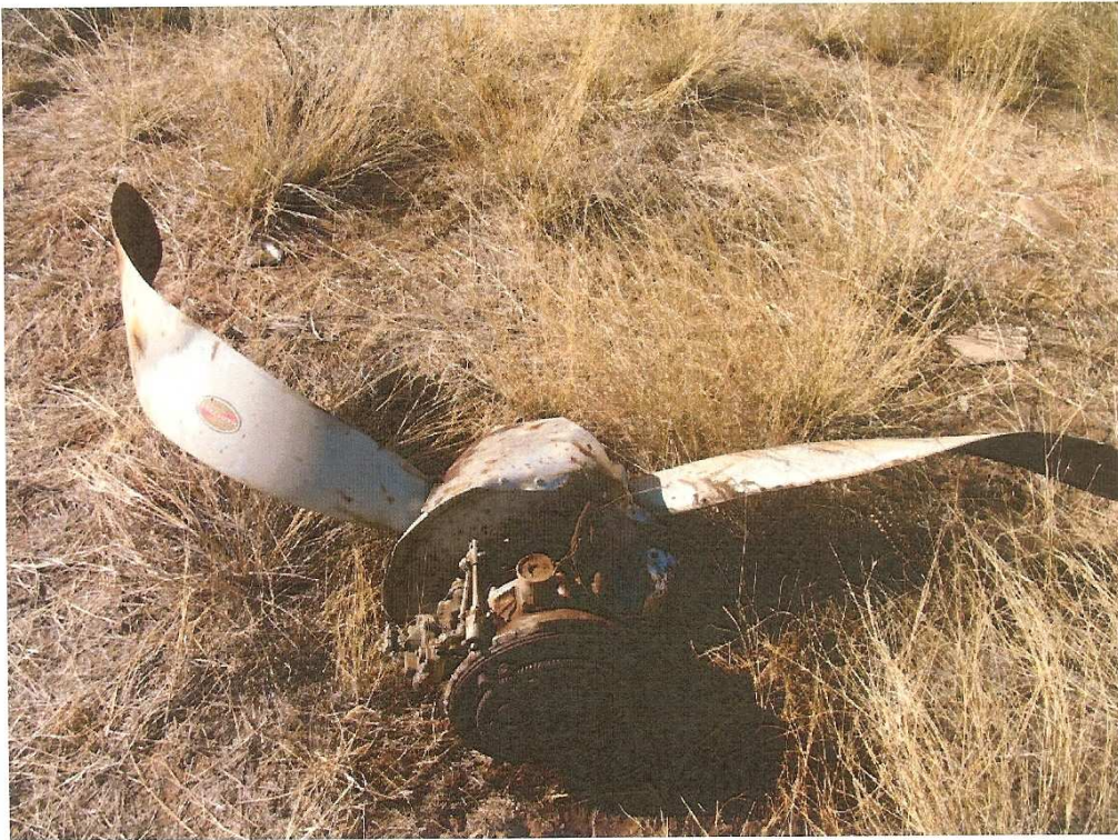
Figure 4: Propeller hub completely disintegrated from the engine a distance away from the main wreckage.
