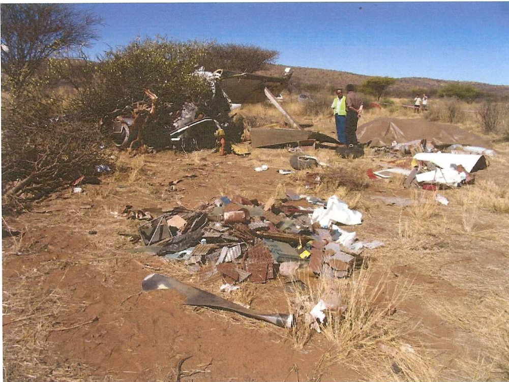
Figure 6: The nose landing gear was broken off from the aircraft and was found a distance from the main wreckage.
