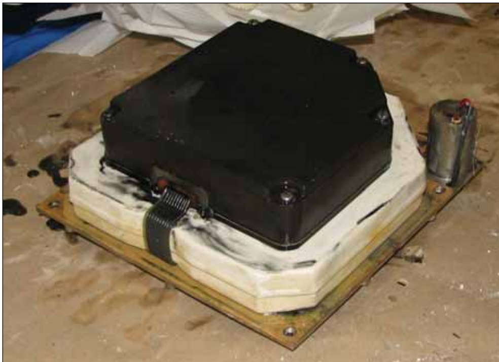
Figure B-24: Crash protected module opened
