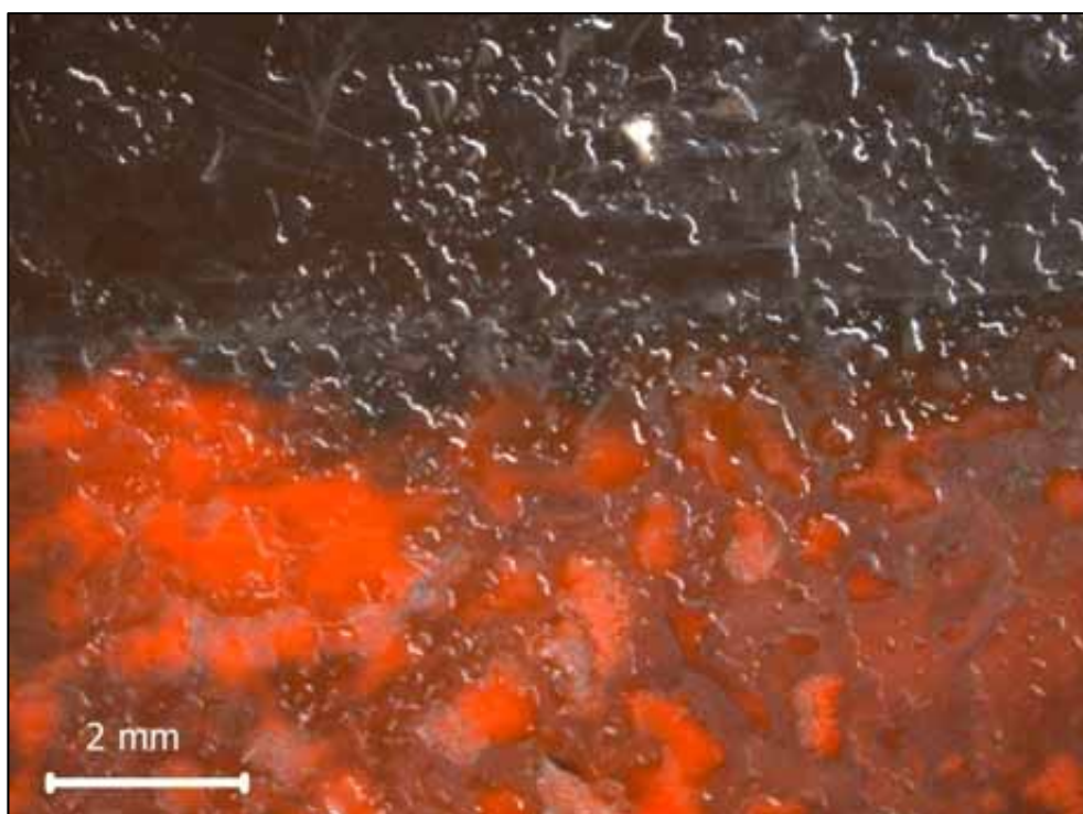
Figure C-4: Magnified view of the discolouration observed on the CVR face plate
