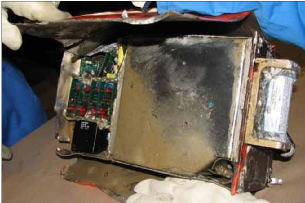
Figure B-24: Crash protected module opened
