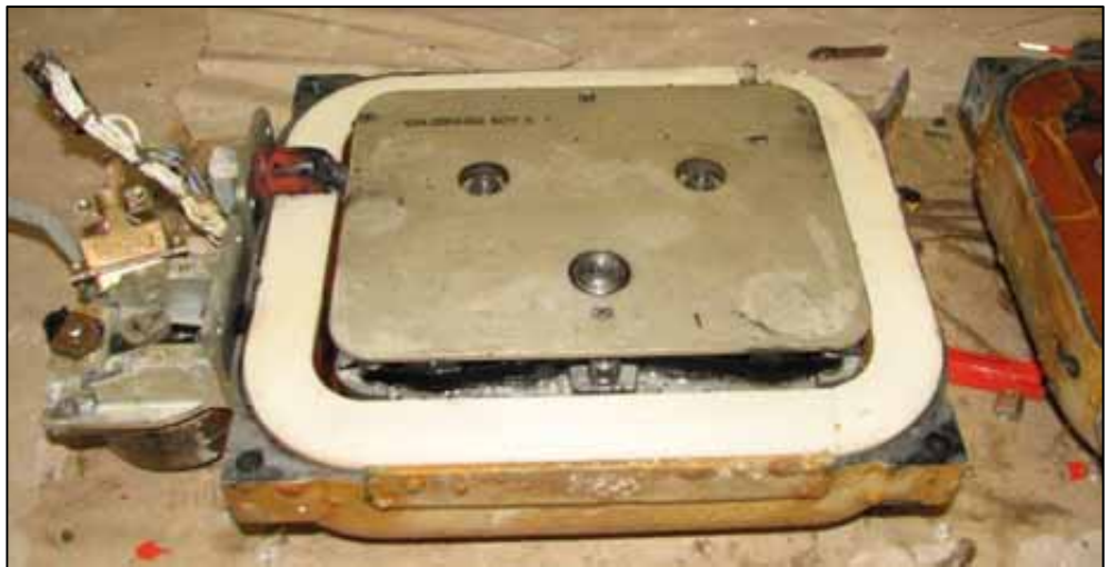
Figure B-9: Crash protected module opened
