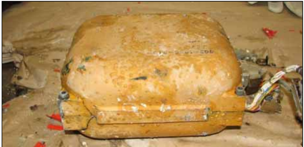
Figure B-9: Crash protected module opened
