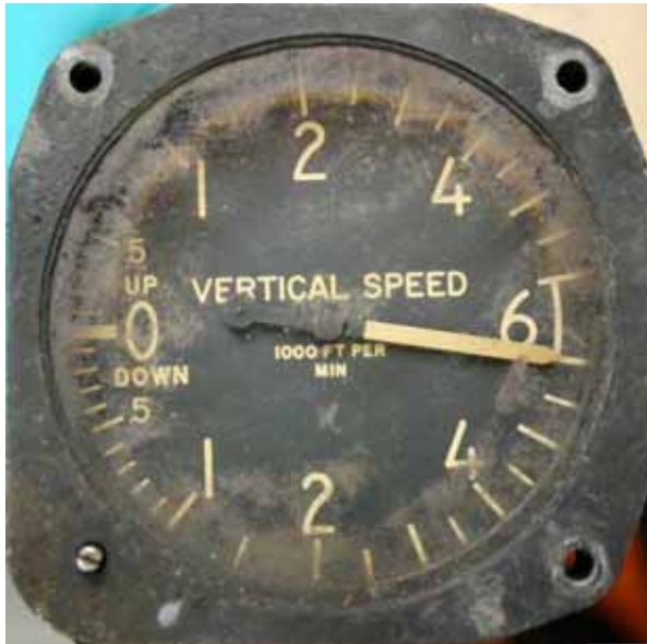
Figure 24: Vertical speed indicator (recovered from VH-TFU)
