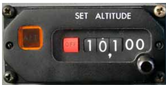
Figure 10: Altitude alerter (Image of representative item, not specific item in VH-TFU)
