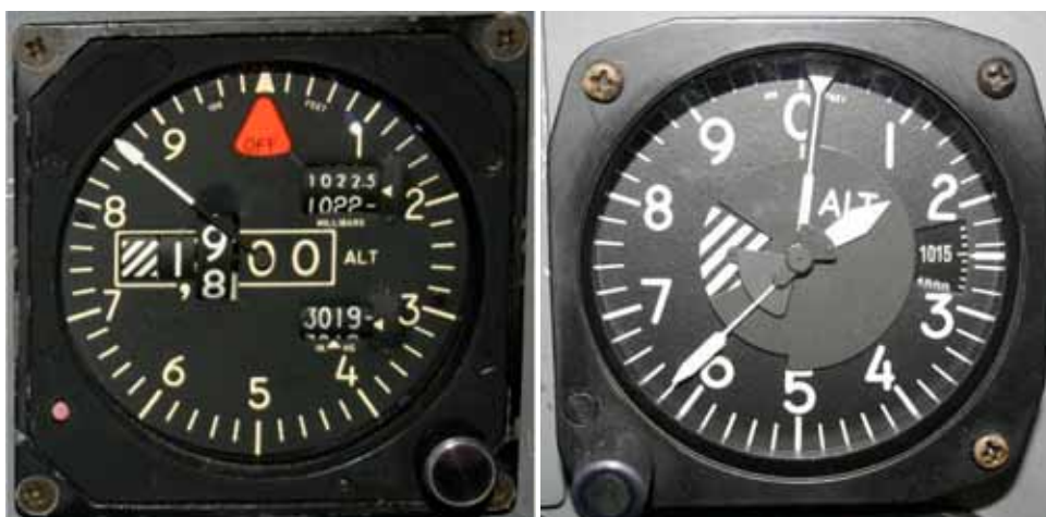
Figure 8: Altimeters - Pilot in command's (left), copilot's (right) (Images of representative items, not specific items in VH-TFU)
