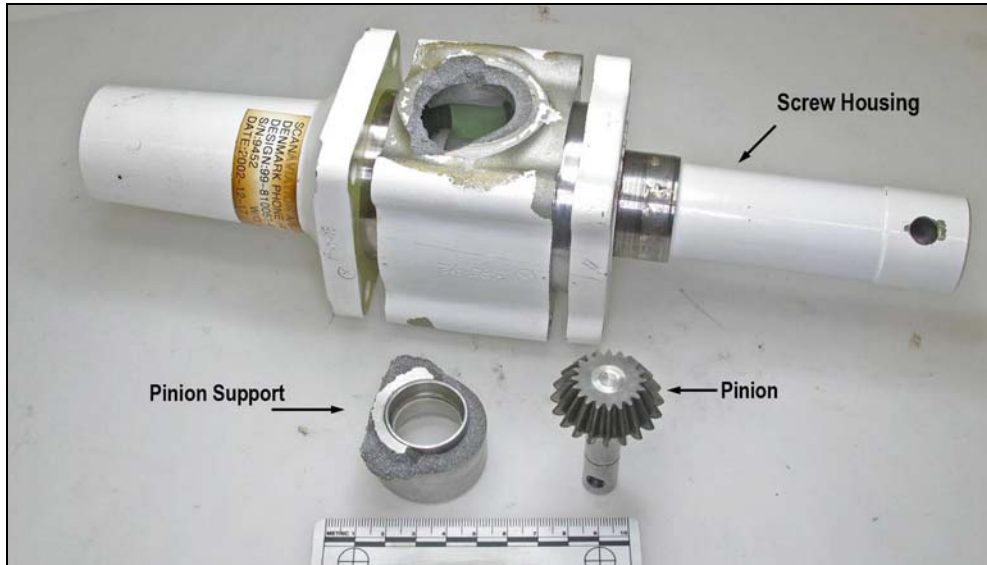
Figure 5: Close view of the mechanical relationship between the pinion and actuator screw.
