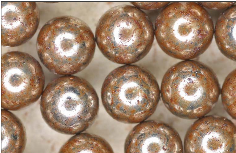
Figure 12: Close-up of the balls from the left bearing showing gross amounts of red contamination over the rolling surfaces.
