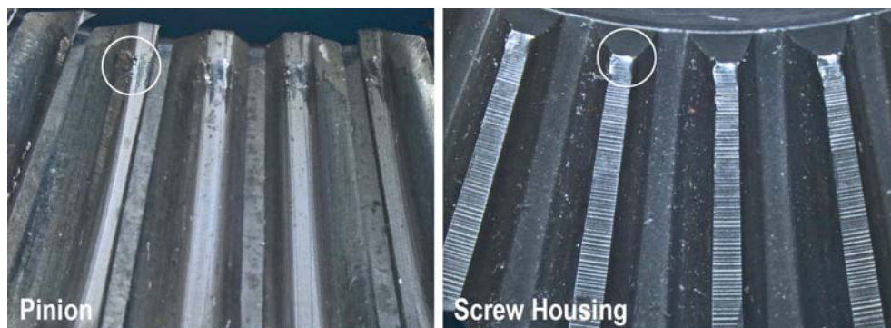
Figure 8: Image montage showing abnormal wear features (circled) on the inner radial meshing teeth off the screw housing and pinion gear.
