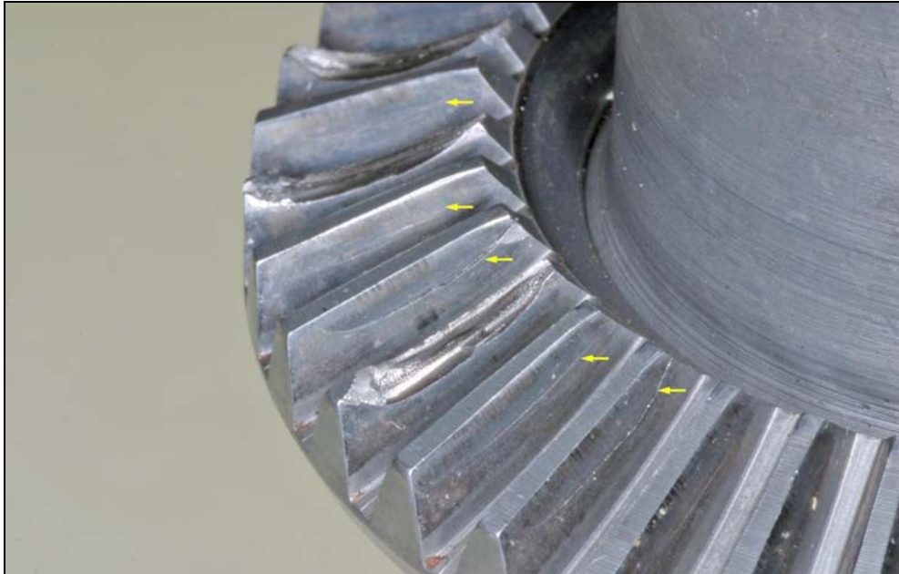
Figure 6: Close-up of the bevelled gear teeth from the screw housing. Note the cracking (arrowed) and tooth loss.
