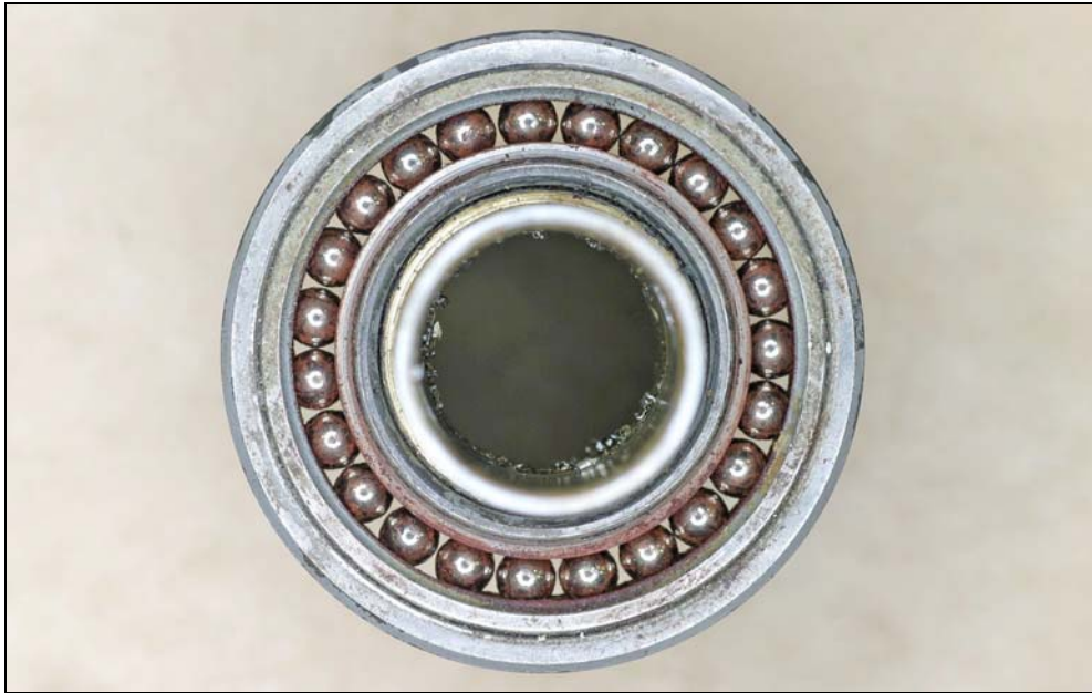
Figure 11: Bearing (P/N KP168S) from the left inboard torque tube support assembly.
