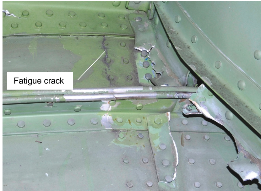
Figure 20. Fatigue cracks seen from the inside of the right wing
