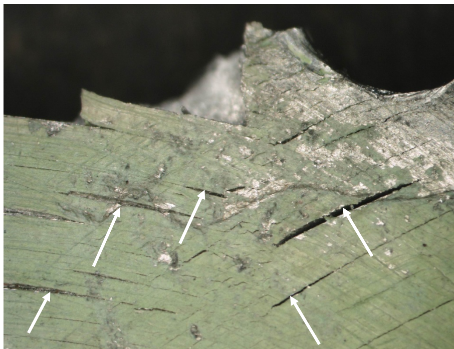
Figure 23. Example of micro-cracks in the finishing
