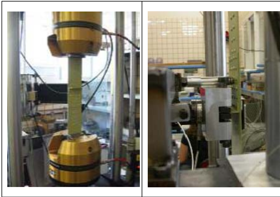
Figure B15. Fatigue test in one load direction
