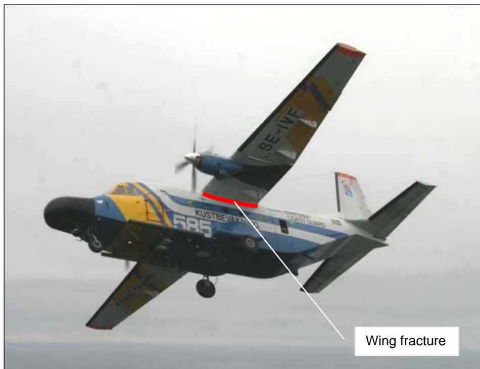
Figure 17. Location of the fatigue cracking
