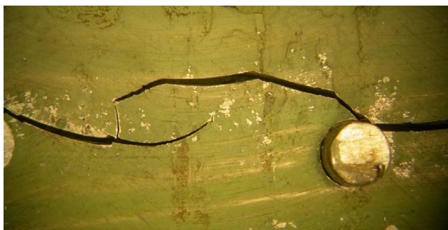
Figure 27. Example of crack growth by “jumping”
