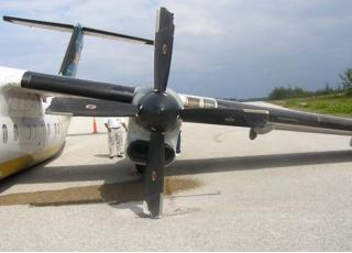
Forward view of Damaged Left Propeller.
