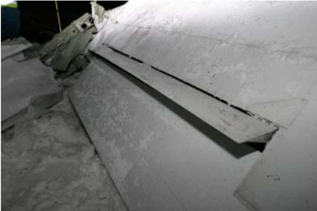
Figure 4. Impurities on the upper wing surface
