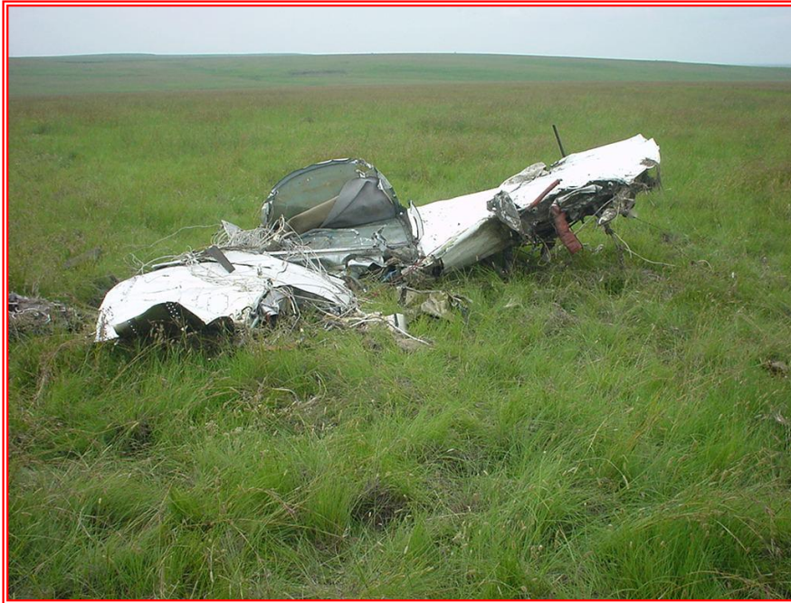
Photo 3: Wing Centre Section viewed from the front & R/H Engine on the left
