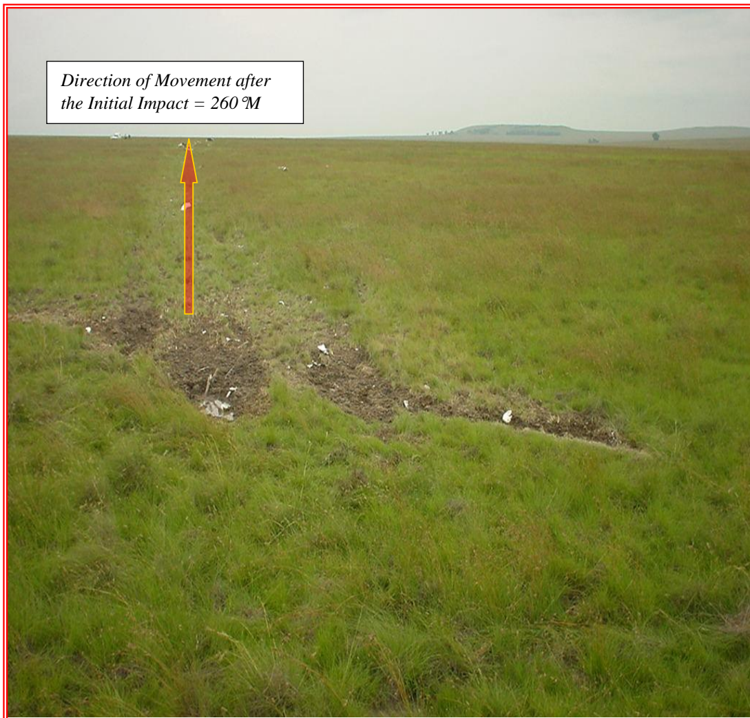
Photo 1: Initial Impact Mark. Heading 260°. It can be seen from the photo that the Aircraft was in a 30° right-wing low attitude during the initial impact.
