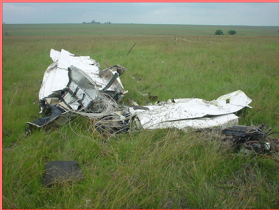
Photo 1: Wing Centre Section viewed from behind and R/H Engine on the right
