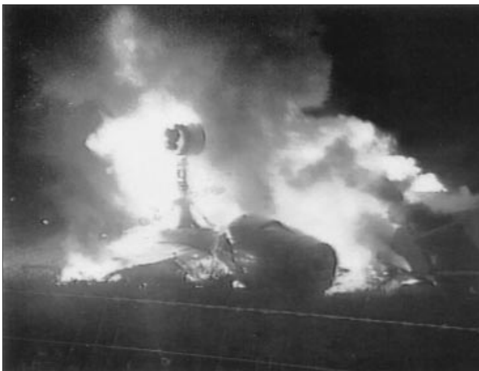
FIGURE 3 Image from video recording, showing the left main landing gear leg extending upwards from the inverted left wing
