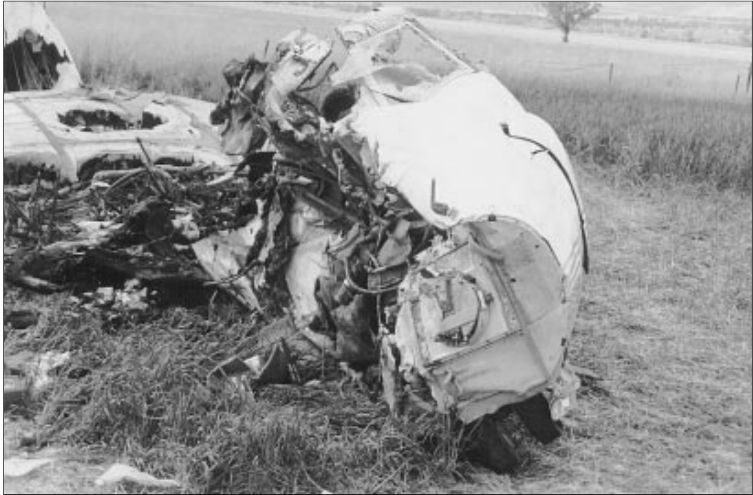
FIGURE 4 Nose section of aircraft, showing impact damage to right side
