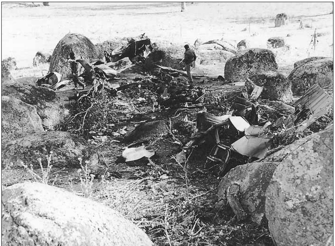
Figure 9 The forward section of the aircraft was totally destroyed by impact forces and fire.
