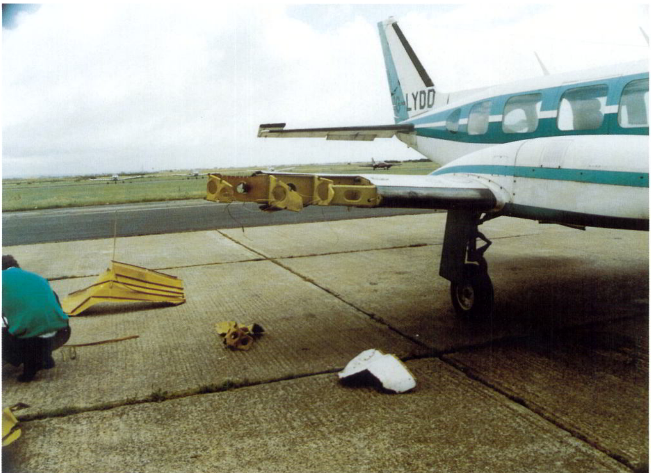
PA-31 G-LYDD View showing damage to right wing
