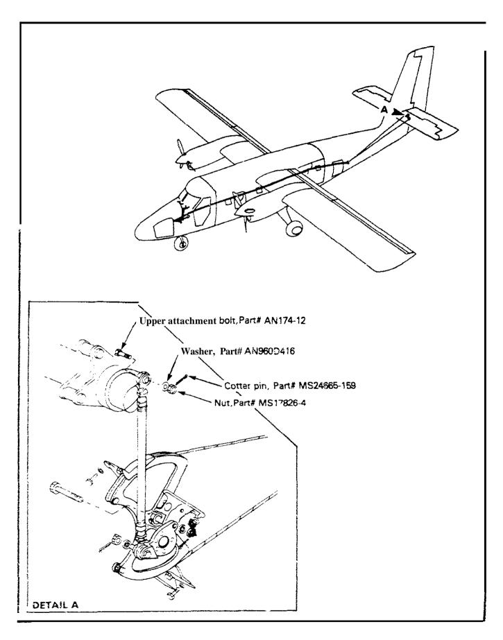
Figure 5.—Elevator control installation, from deHavilland DHC-6-300 PC, Chapter 27-30-00, page 0, figure 1 (descriptions added to the illustration for clarity).
