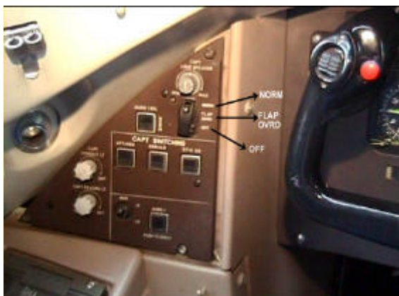
Figure 5 : Three-position GPWS switch in NORMAL position
