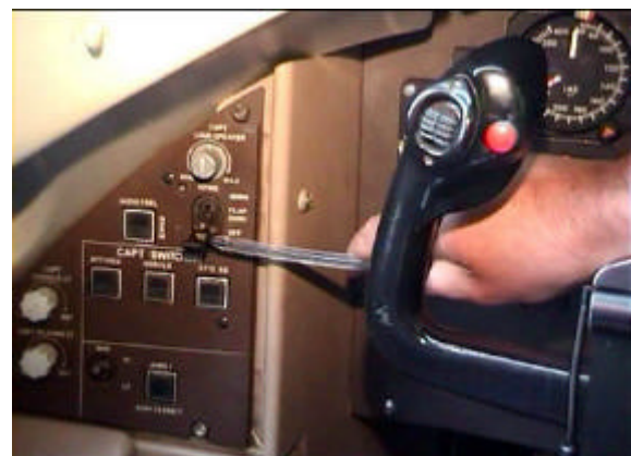
Figure 6 : Three-position GPWS switch in OFF position
