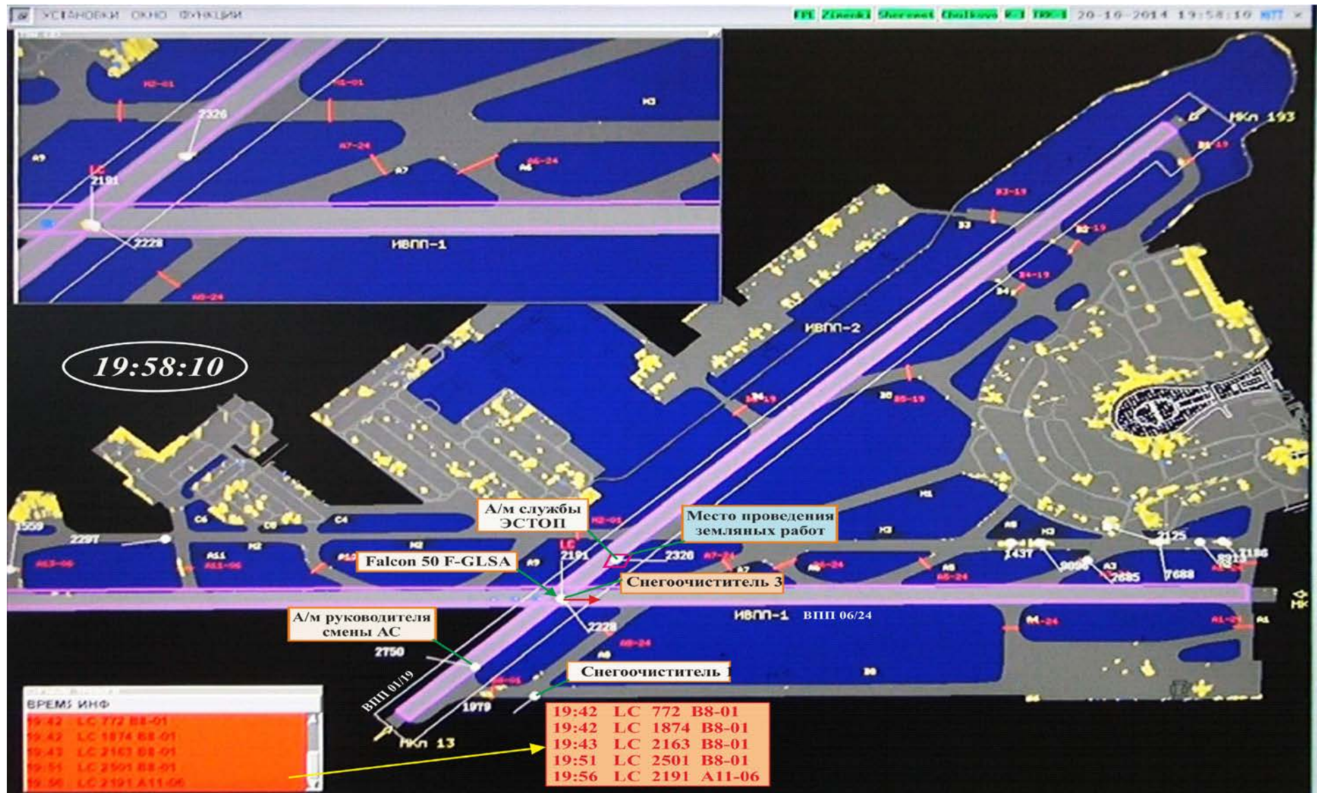
Figure 86. Location of objects at airdrome Vnukovo as viewed from the departure controller screen at 19:58:10 during the Falcon-50EX F-GLSA aircraft collision with snowplow 3
