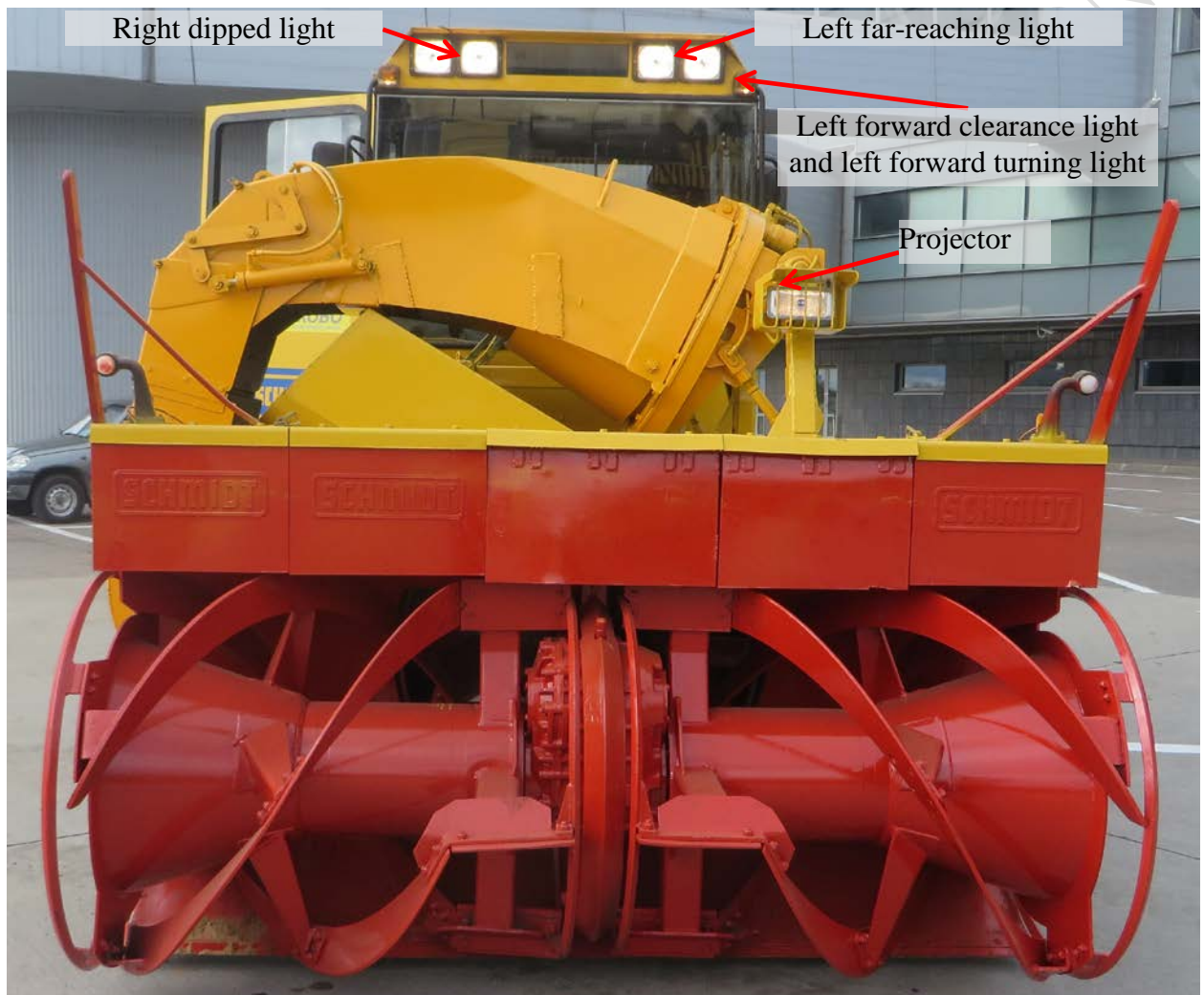
Figure 46b. Snowplow lights schematic (forward)
