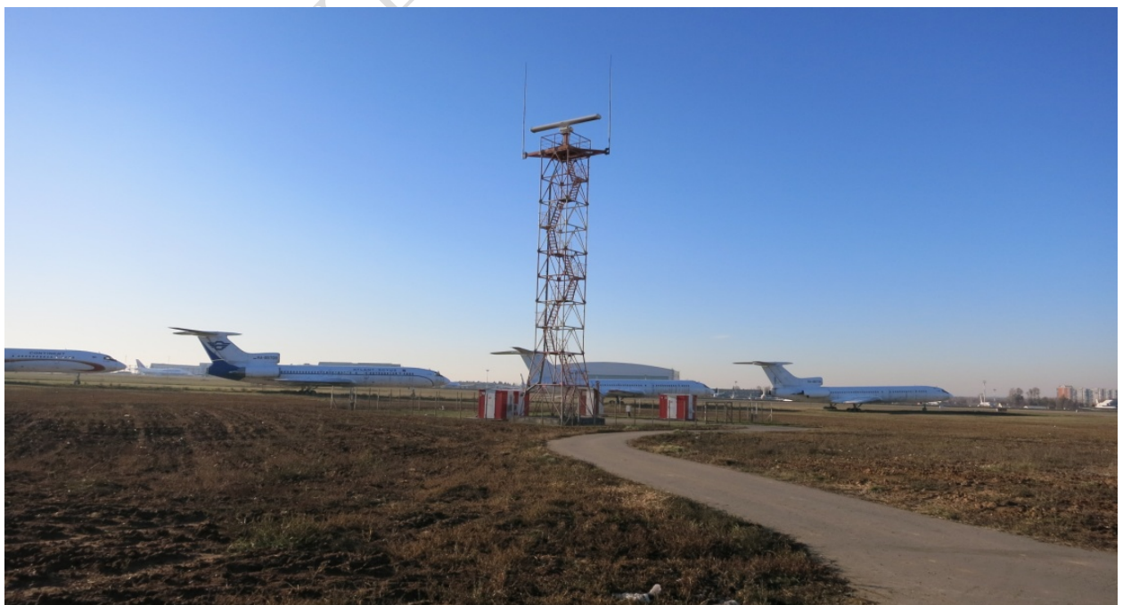
Figure 4. General view of the airfield surveillance radar at Vnukovo airdrome
