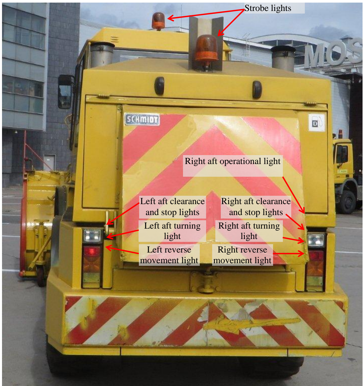
Figure 46c. Snowplow lights schematic (aft)
