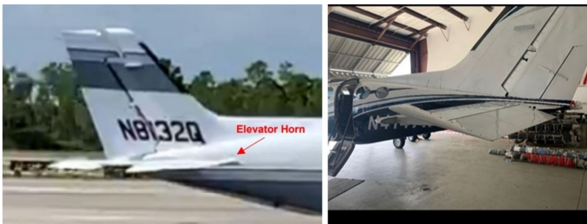
Figure 1 – Still frame from video footage of the accident airplane's elevator during taxi (left) compared to the elevator on an exemplar airplane with a control lock installed (right).
