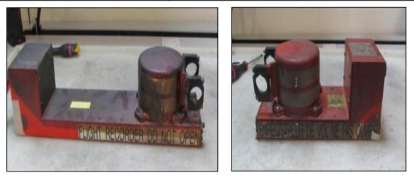
Figure: 1-26 Digital Flight Data Recorder
