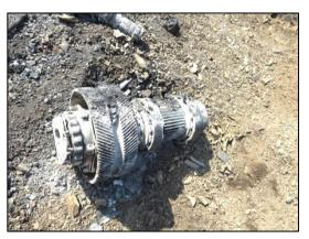
Figure: 1-63 Figure: 1-64 Gear Trains Detached from Main RGB Assemblies
