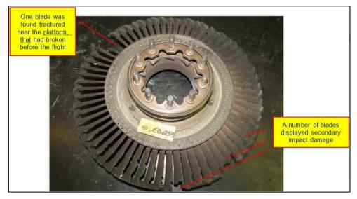
Figure 1-3: Power Turbine Stage 1 (PT-1) One Blade Fractured
