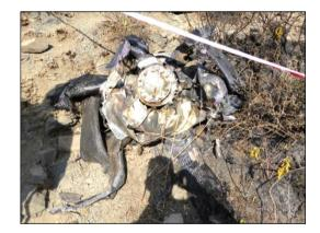
Figure: 1-45 No 1 Propeller with Blades Installed and No 1 Propeller Blades Damaged due to Signs of Ground Fire
