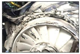
Figure: 1-56 No 1 Engine Impeller – No Damage
