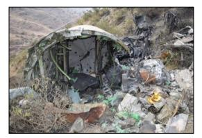
Figure: 1-32 Rear Fuselage Detached on Impact
