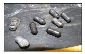
Figure 2-7 : No 6 Bearing Rollers
