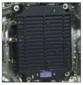
Figure 1-93: Electronic Engine Control
