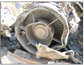
Figure: 1-62 No 2 Engine Power Turbine - No Damage
