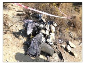
Figure: 1-47 No 1 Propeller Blades Damaged due to Post Impact Fire
