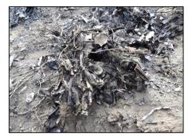
Figure: 1-44 Burnt Electrical Looms and Parts
