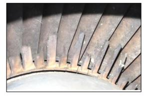
Figure: 1-55 Power Turbine 2 Damaged Blades (Closer View)
