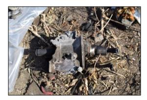
Figure: 1-35 Propeller Valve Module (PVM)
