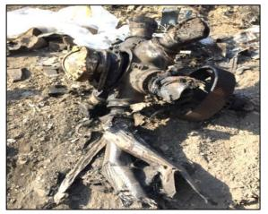
Figure: 1-50 No 2 Propeller with Blades Detached on Impact
