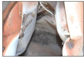
Figure: 1-59 View of Tail Pipe - Sign of Metallization in Folds (Brownish Color)
