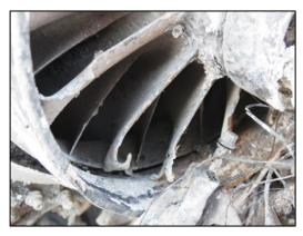
Figure: 1-60 No 2 Engine LP Impeller – Blades Bent Opposite to Direction of Rotation
