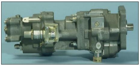
Figure 1-4: Serviceable Overspeed Governor (OSG)
