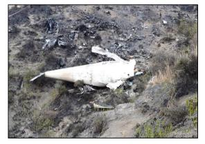
Figure: 1-29 Rear Fuselage and Structural Parts
