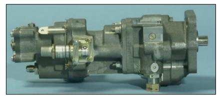
Figure 1-103: OSG and the Main Pump
