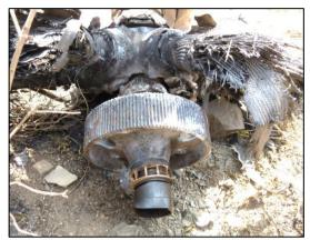
Figure: 1-48 Bull Gear of RGB Attached with No 1 Propeller
