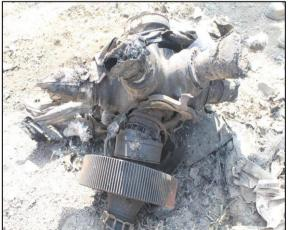
Figure: 1-51 Bull Gear of RGB Attached with No 2 Propeller
