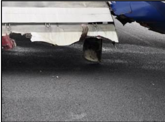
Figure 7: Shows damage on the trailing edge flaps
