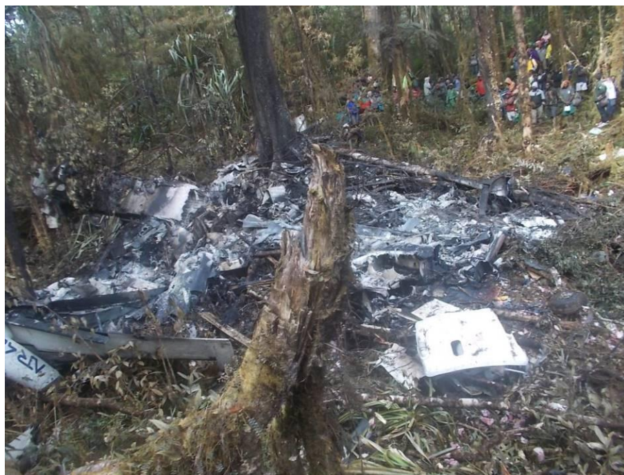
Figure 8: The wreckage of the fuselage damaged by post-impact fire
