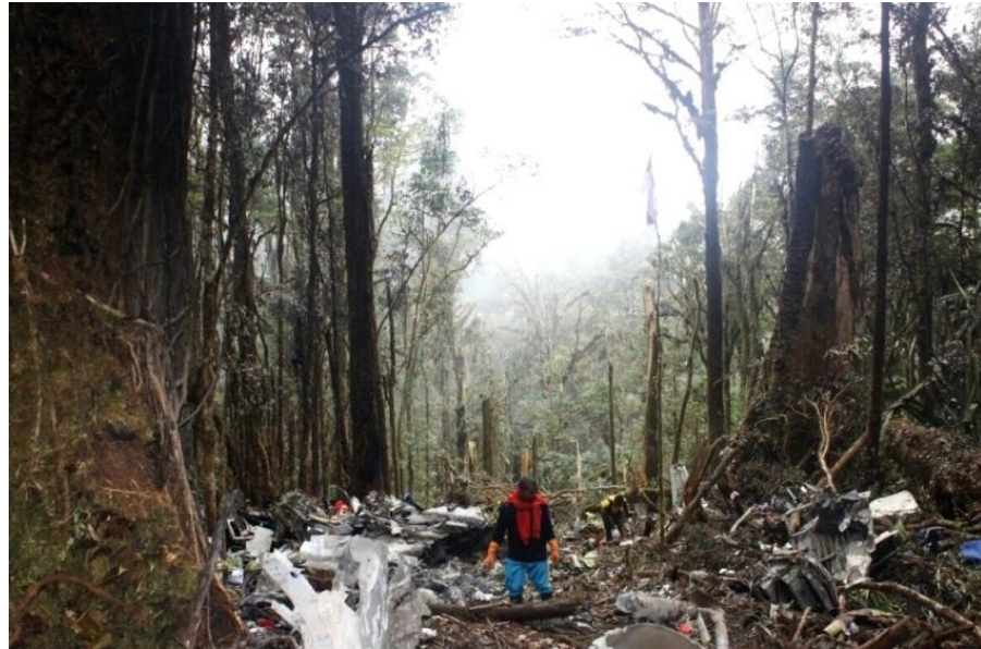
Figure 7: The view from the accident side toward the aircraft flight path showed opening forest trees that likely caused by impact to the aircraft
