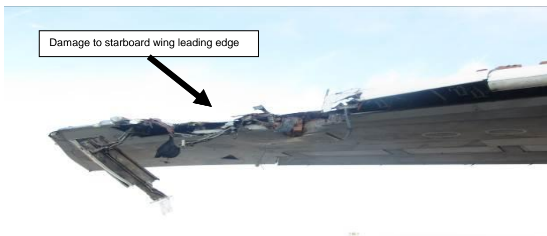
Figure 40 Damage caused to wing leading edge
