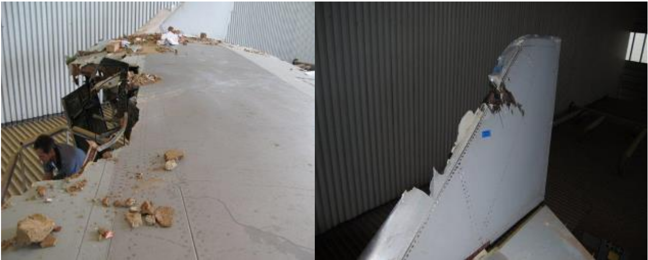
Figure 41 Damage caused to wing upper skin structure and winglet
