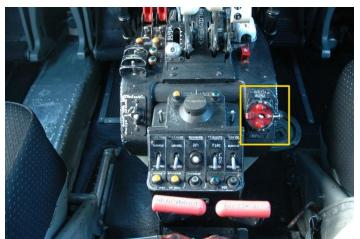
The landing gear control is located out of the field of view of the pilots and therefore are operations not observable by the captain and first officer, specifically during take-off and landing, when both pilots are engaged with forward view and instrument scan.
