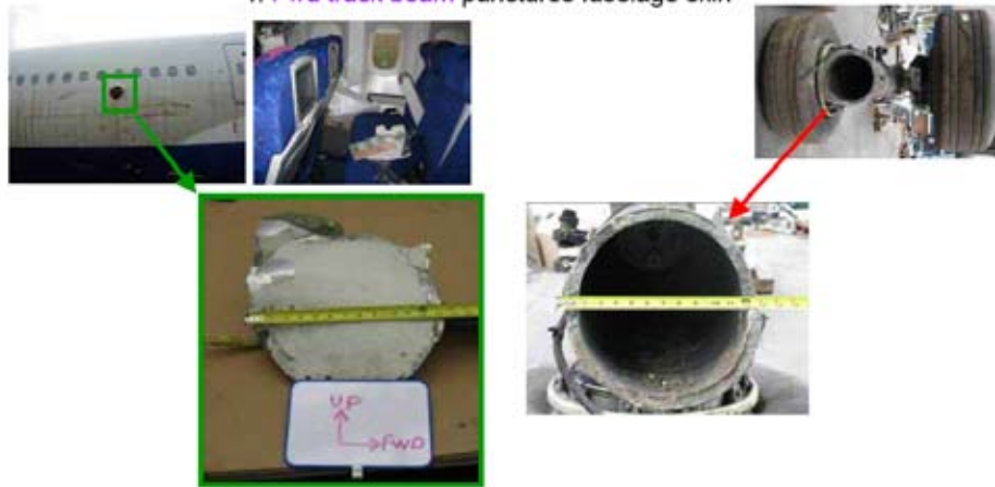
4. Fwd truck beam punctures fuselage skin
