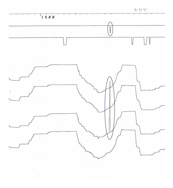
Flight Data Recorder graphs from the previous flight (Trondheim to Namsos). The sudden peak on the performance graph for engine number two (E2TORQ) and the coincident peak on the radio no. 2 (VHF2) are circled in.
