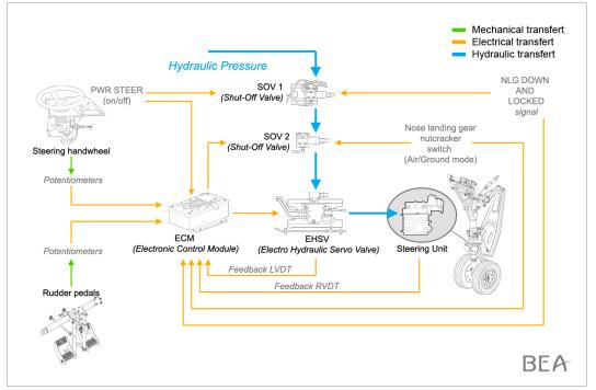
Figure 5: nose gear steering control system
