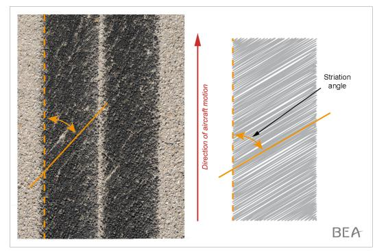
Figure 13: striations observed on the nose gear marks and method for measuring the angle
