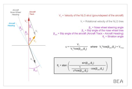
Figure 24: diagram of speed composition
