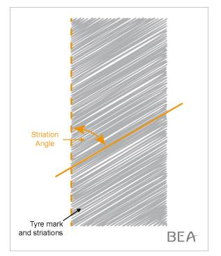
Figure 2: convention for measuring the striation angle
