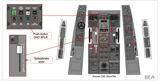
Figure 6: GND SPLR push-button and speedbrake control
