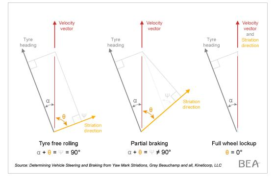
Figure 21: orientation of the striations for a braked wheel and an unbraked wheel, schematic diagram
