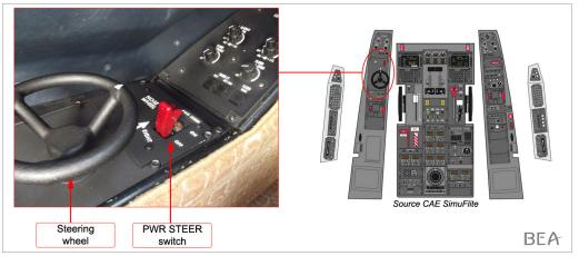
Figure 4: tiller and guarded PWR STEER switch
