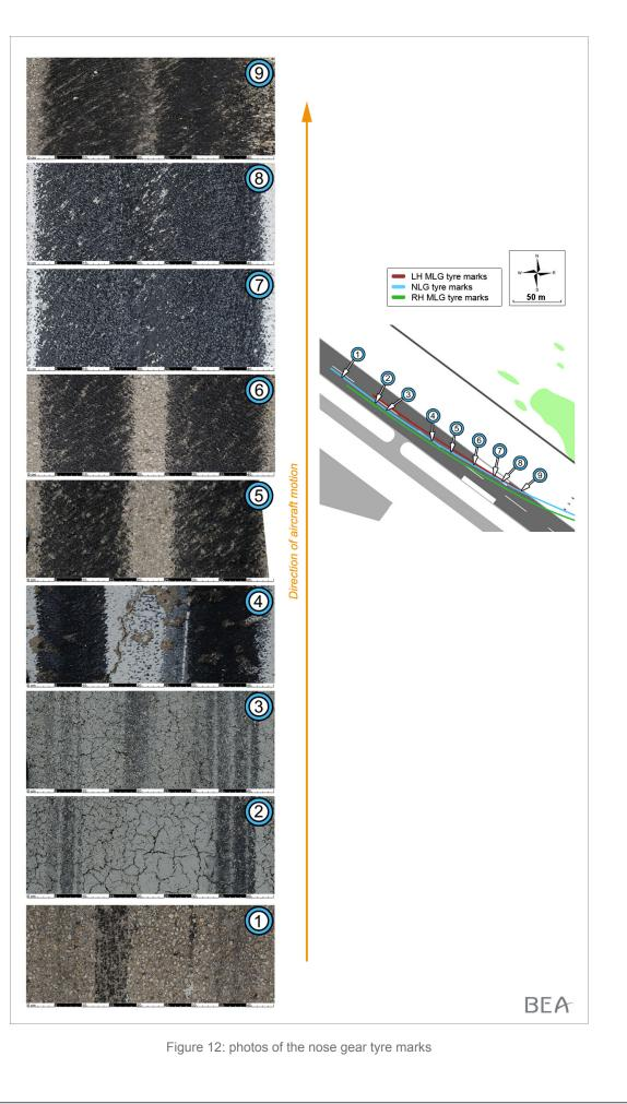
Shortly before the runway centre line (between points 3 and 4 of the diagram above) and until the runway edge these marks had striations trending towards the right in the direction of travel of the aeroplane. Their angle, measured between the edge of the mark and the striation, changed along the marks (see the measurements below).
