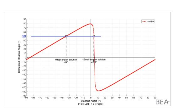
figure 26: example of a striation angle value in relation to wheel orientation, for wheel rotation speeds close to their theoretical maximum value (u = 0.99) with a 5° right sideslip
