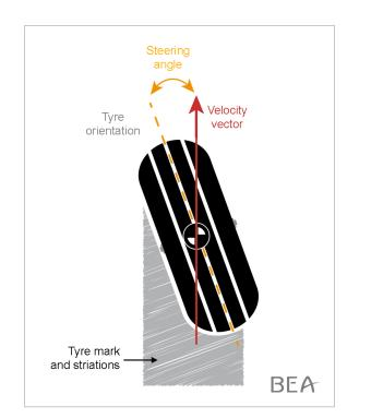
Figure 23: orientation of striations during tests, schematic diagram
